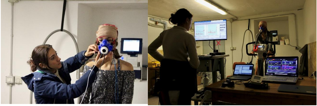
Figure 9. Experimental setup for the breath-by-breath measurements of gas exchange employed both at rest and during exercise.
