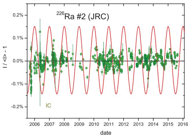
**Figure 15.** Residuals from exponential decay for  $^{226}\text{Ra}$  (source #2) activity measurements with the IG12 IC of the JRC.
