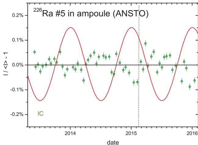
**Figure 26.** Residuals from exponential decay for  $^{226}\text{Ra}$  (source #5 in an ampoule) activity measurements with the IC of ANSTO. The dotted line marks the installation of a new electrometer.
