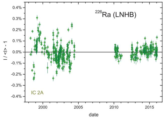
**Figure 36.** Residuals from exponential decay for  $^{226}\text{Ra}$  activity measurements with the IC 2A of LNHB.
