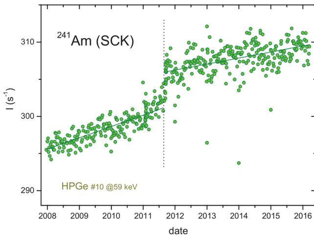
**Figure 46.** Decay-corrected net peak count rates at 59 keV from the decay of  $^{241}\text{Am}$  measured with HPGe detector #10 at the SCK•CEN. The dotted line marks a change of data acquisition system and the full lines represent linear trend lines.
