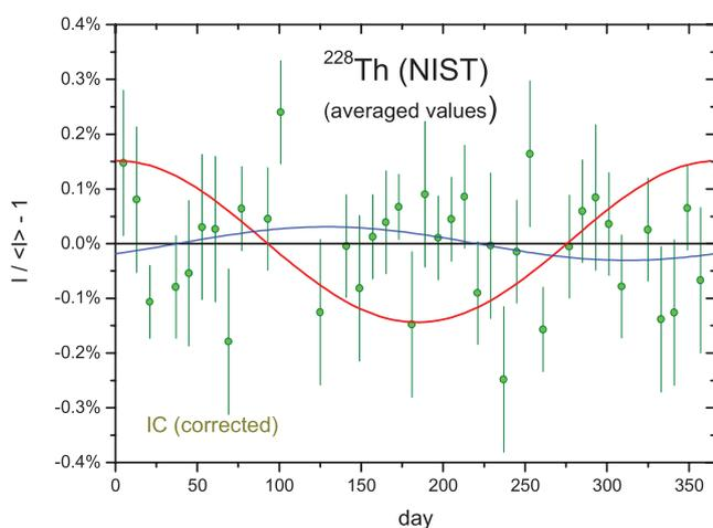
**Figure 55.** Annual average residuals from exponential decay for  $^{228}\text{Th}$  decay rate measurements with IC 'A' at NIST, after minor corrections for geometrical instability of the source holder.
