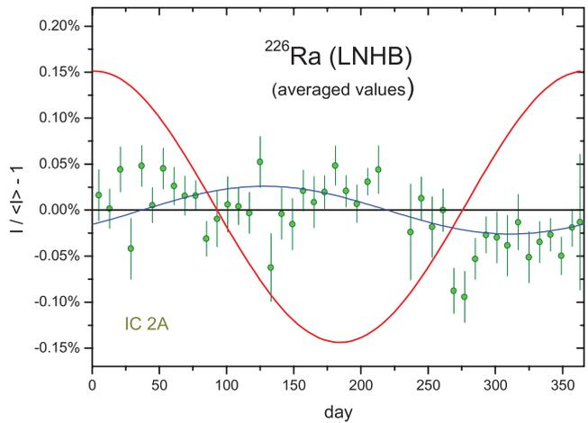
**Figure 37.** Annual average residuals from exponential decay for  $^{226}\text{Ra}$  activity measurements with the IC 2A of LNHB.
