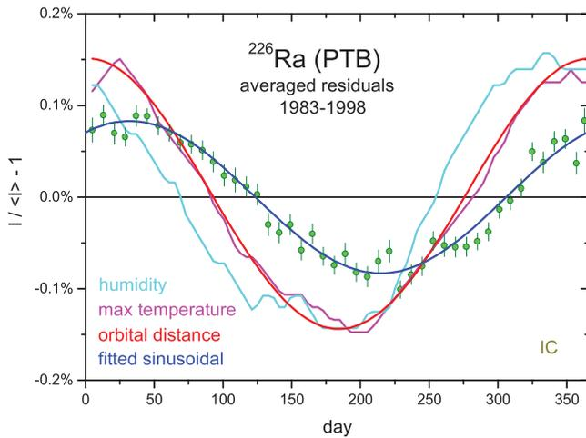
**Figure 2.** Annual averages of the residuals in figure 1 for periods of 8 d, compared to renormalised relative changes in  $1/R^2$  for Earth–Sun distance as well as in the outdoor humidity and maximum temperature in the Braunschweig area. The sign of the temperature data was reversed to facilitate direct comparison.
