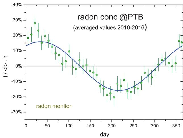
**Figure 3.** Annually averaged relative variations of radon concentration in the air inside the PTB laboratory room where the IC is installed, measured with a radon monitor from mid 2010 up to mid 2016. The line represents a sinusoidal function fitted to the data. The annual oscillations in radon concentration appear to be in phase with the modulations of the  $^{226}\text{Ra}$  ionisation current in figure 2.
