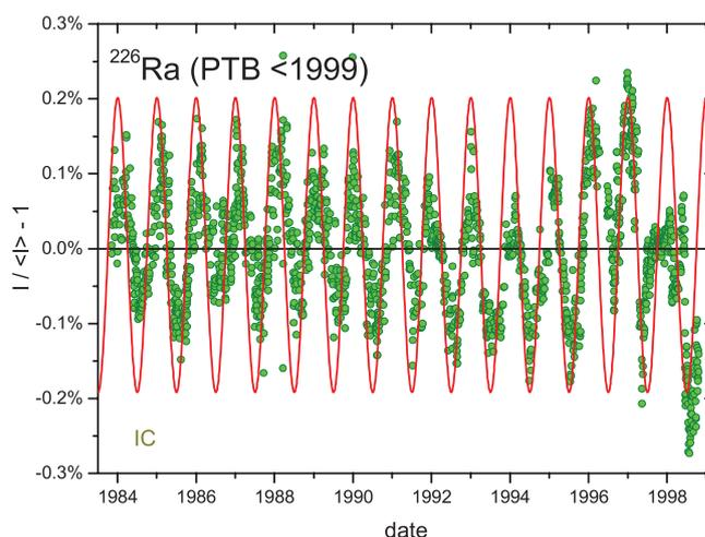
**Figure 1.** Residuals from an exponential decay curve of the ionisation current from a  $^{226}\text{Ra}$  source inside the IG12/A20 ionisation chamber at PTB measured between 1984 and 1998. The line represents relative changes in the inverse square  $1/R^2$  of the Earth–Sun distance, normalized to an amplitude of 0.2%.
