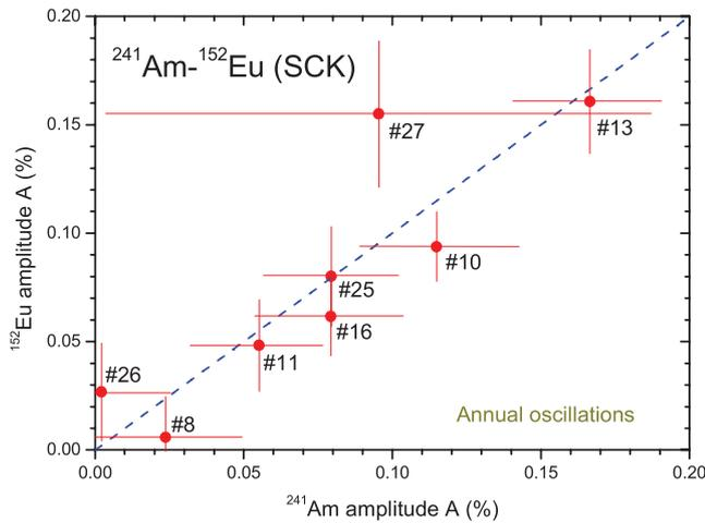
**Figure 50.** Amplitude of average annual oscillations in the decay rate of  $^{241}\text{Am}$  and  $^{152}\text{Eu}$  measured by  $\gamma$ -ray spectrometry with 8 detectors at SCK between 2008 and 2016.
