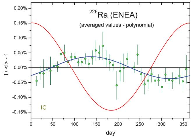
**Figure 9.** Annual average residuals from exponential decay for  $^{226}\text{Ra}$  activity measurements with the ENEA IC, in which the input data were first detrended by means of the trend line in figure 8.
