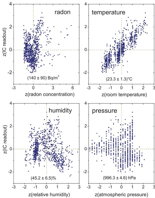
**Figure 10.** Correlation plot of averaged  $^{226}\text{Ra}$  current readouts in the ENEA IC with radon concentration in air, room temperature, relative humidity and atmospheric pressure measured from March to May 2016 in the ENEA laboratory. The data were rescaled to a z-score using  $z = (x - \mu)/\sigma$ .
