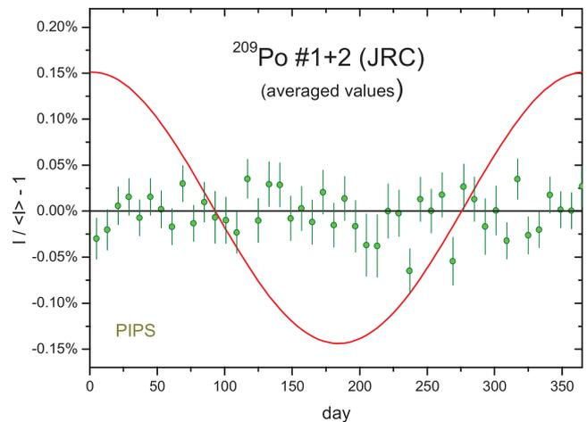
**Figure 41.** Annual average residuals from exponential decay for  $^{209}\text{Po}$  activity measurements with a planar silicon detector at JRC.
