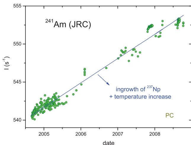
**Figure 42.** Measured count rate from photon (and electron) emission in the decay of  $^{241}\text{Am}$  with a gas-filled proportional counter in fixed low solid angle geometry at JRC.
