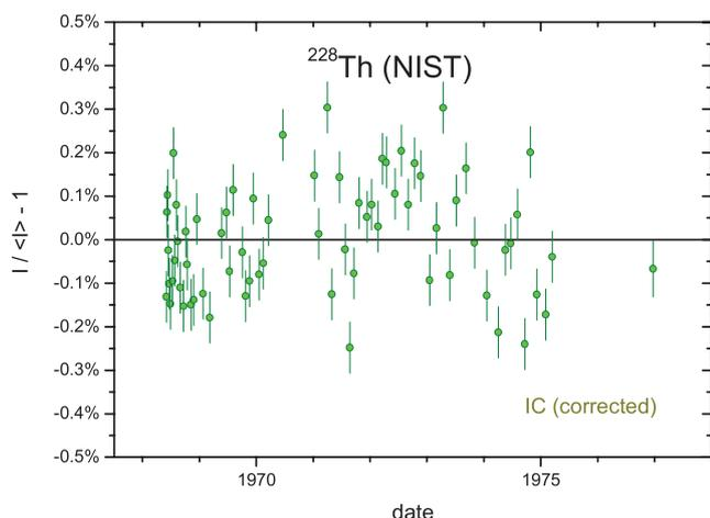
**Figure 54.** Annual average residuals from exponential decay for  $^{228}\text{Th}$  decay rate measurements with IC 'A' at NIST, after minor corrections for geometrical instability of the source holder.
