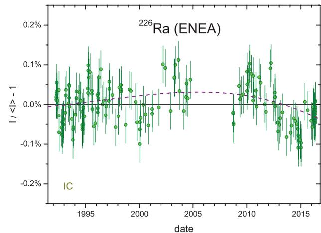
**Figure 8.** Residuals from exponential decay for  $^{226}\text{Ra}$  ionisation current measurements with the IG11 IC at ENEA between 1992 and 2016. The dashed line shows a trend line fitted to the data.
