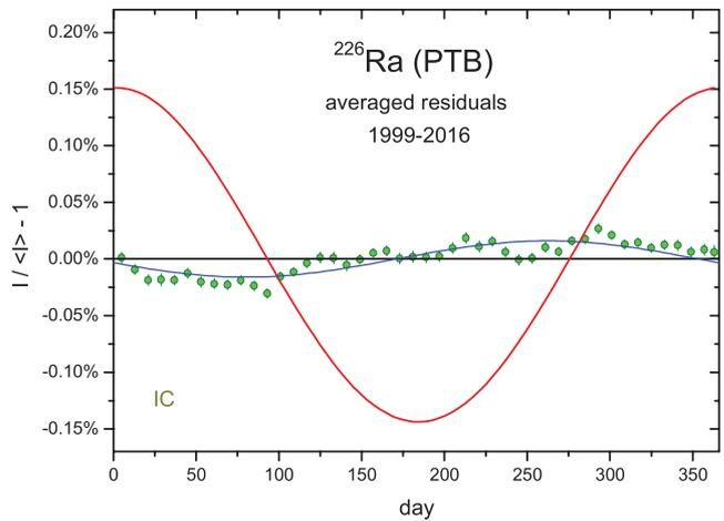
**Figure 5.** Annual average residuals from exponential decay for  $^{226}\text{Ra}$  ionisation current measurements with the PTB IC from 1999 to 2016. The modulations are smaller than in figure 2 due to a replacement of electronics.
