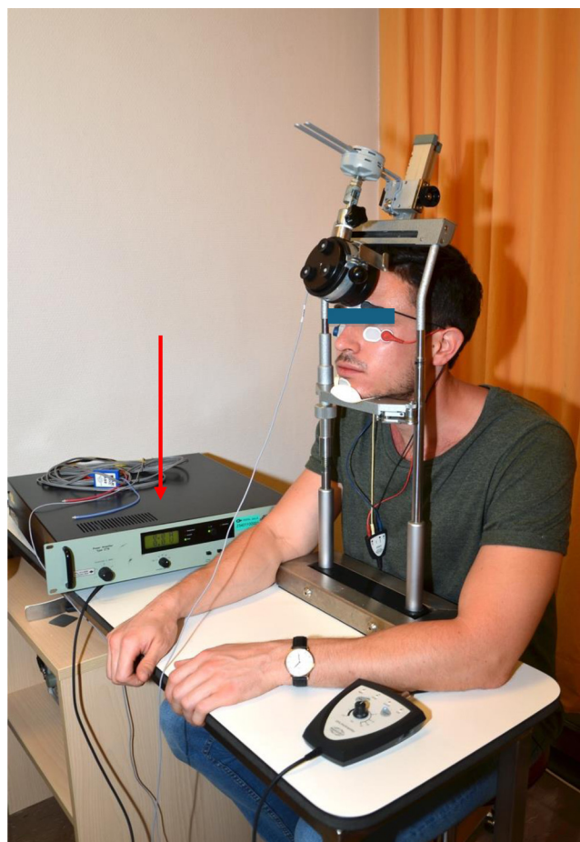
Fig. 2. Frontal stimulation. Modified slit lamp holding the bone vibrator and allowing a three-dimensional adjustment of the position of the bone vibrator on the patient's forehead. The small digital display on the Brüel and Kjær amplifier type 2718 (red arrow) showed the electrical current delivered by the device according to the pressure applied, allowing the optimal pressure on the forehead to be adjusted.
