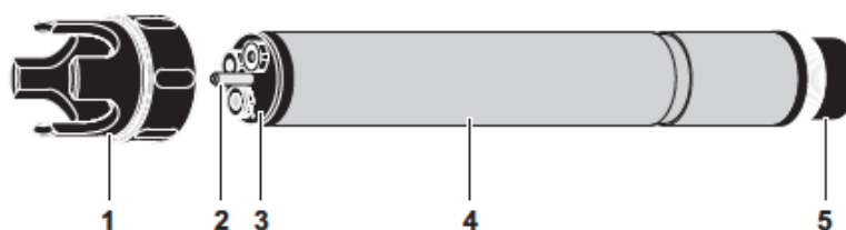
Figure 3: Illustration of the ion-selective electrode used to measure ammonium online (AmmonLyt® Plus 700IQ, WTW GmbH, Weilheim, Germany). 1) Protective hood, 2) Temperature probe, 3) Support and electrodes, 4) Sensor shaft and 5) Plug head connection. Reproduced with the kind permission of WTW GmbH, Weilheim, Germany (AmmonLyt® Plus 700IQ, user manual, fig. 1-2, page 1-2).
