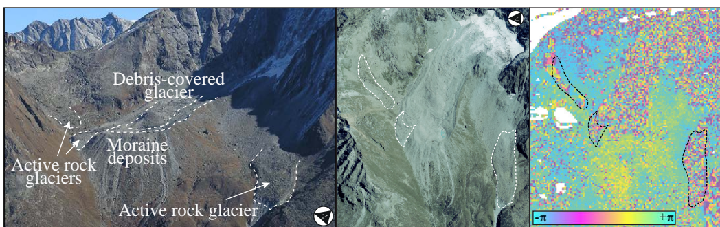
Fig. 3.4.: The rock glaciers of the Tsarmine sector (left) and their mapping by ortho-image interpretation (center; orthophoto: swisstopo). Right image illustrates the InSAR signal between 23/07/2009 and 08/10/2009.
