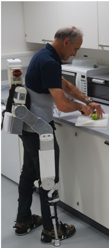
Fig. 1 Illustration of a powered lower limb exoskeleton actuated at the level of the hip and knee joints. It assists the abduction/adduction and flexion/extension of the hip joint, and the flexion/extension of the knee joint (LLE Autonomy, [12, 13])
