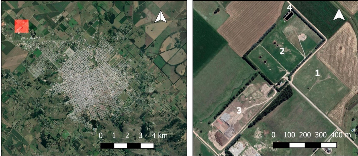
Figure S2. Location of the sanitary landfill (left). At the right: 1) the old open dump; 2) the first landfill (1998-2013); 3) the new sector (2104-2021?); 4) the leachate plant. Image source: Google Maps.
