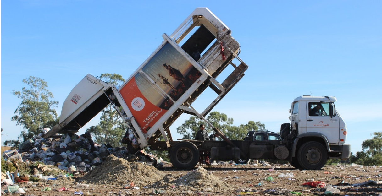
Figure 37: A new compactor truck downloading waste in the sanitary landfill in 2016. Photo credit: the author
