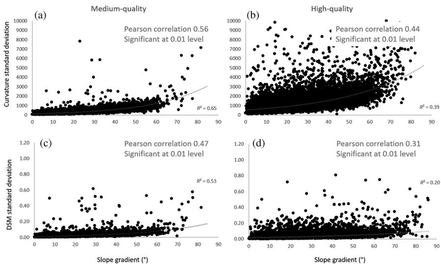
**Figure 6.** The exponential relationship between slope gradient and the variation in curvature (a, b) and the variation in DSM ( $z$ ) (c, d) for both medium- and high-quality runs, where the number of overlapping pictures is at least five. With  $R^2$  as the coefficient of determination.
