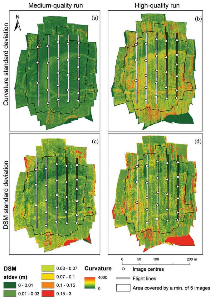
**Figure 4.** Standard deviations of the curvature value of each cell for the ten model runs in medium- (a) and high-quality run (b) and of the DSM value in  $z$  of each cell for the ten model runs in medium- (c) and high-quality run (d).
