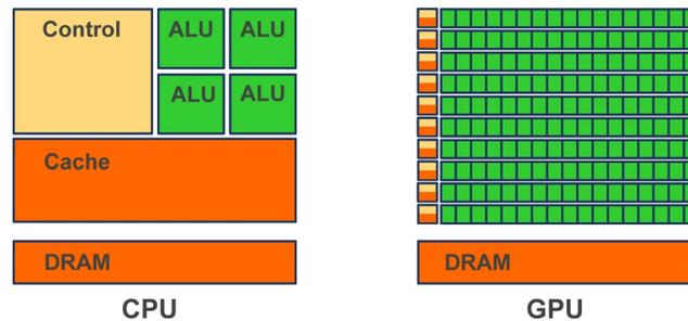
**Figure F1.** Schematic chip representation for both the central processing unit (CPU) and graphical processing unit (GPU) architectures. The GPU architecture consist of thousands of arithmetic and logical units (ALU). On the CPU, most of the on-chip space is devoted to controlling units and cache memory, while the number of ALUs is significantly reduced.
