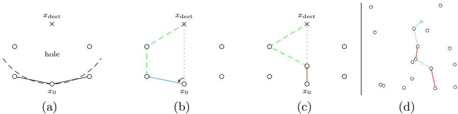
**Fig. 1.** Illustration of a *routing hole* in a WSN. (a) Node  $x_0$  is closer to the destination  $x_{dest}$  than its neighbors making greedy routing fail. (b) Face-based routing algorithms route along the edges bordering the void while (c) Grasp leverages the node mobility to move toward the destination until greedy forwarding is possible. (d) Sample path using GRASP. Dashed lines denote *greedy forwarding* and solid lines and arrows denote respectively hole circumventing and moving.
