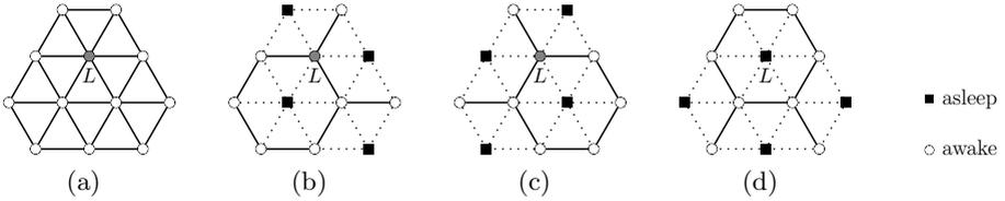
**Fig. 6.** Sleep-Wakeup scheme: (a) nodes inside a triangular lattice adopt in a cyclic manner three sleep-wakeup policies (b),(c) and (d). For the sake of readability, the leader  $L$  is reported in the three figures as a reference point. In each configuration, one third of the nodes are asleep and the communication graph is an hexagonal lattice.
