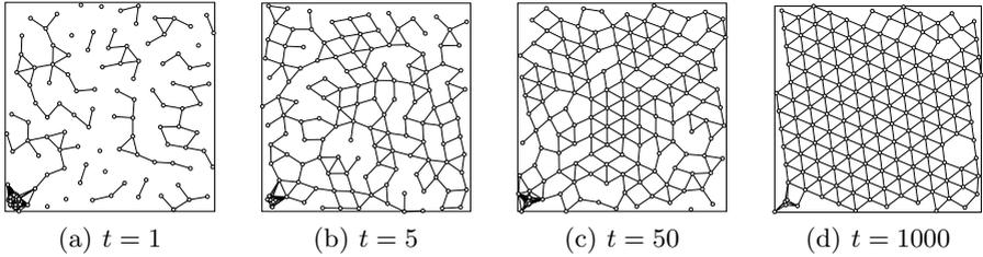
**Fig. 4.** Evolution of the network topology over time. A hundred nodes are initially uniformly deployed on a small area (1/100th) of a 2D toric ROI. The message emission rate is set to  $\lambda = 10$ . The plain lines represent the communication graph. For the sake of simplicity, edges between border vertices are not represented. Note the existence of an hexagonal tile and a few square tiles in the communication graph.
