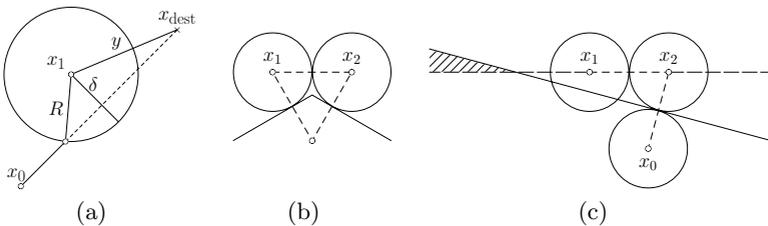
**Fig. 3.** Repulsion radius and attraction sites: (a) two nodes running GRASP cannot get closer than  $\delta = \frac{\sqrt{3}}{2} R$ ; (b) the two points which forms, together with  $x_1$  and  $x_2$ , an equilateral triangle are attraction sites where a node does not need to move to route a message behind the line  $(x_1x_2)$ . (c) Routing toward a destination in the hatched area forces  $x_0$  to move. Plain lines delimit the Voronoï region associated to the nodes.
