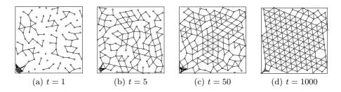
Fig. 4. Evolution of the network topology over time. A hundred nodes are initially uniformly deployed on a small area (1/100th) of a 2D toric ROI. The message emission rate is set to  $\lambda=10$ . The plain lines represent the communication graph. For the sake of simplicity, edges between border vertices are not represented. Note the existence of an hexagonal tile and a few square tiles in the communication graph.
