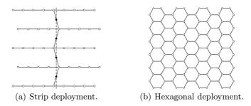
Fig. 2. Node deployments ensuring (a) asymptotically optimal connected-coverage and (b) optimal greedy connected-coverage
