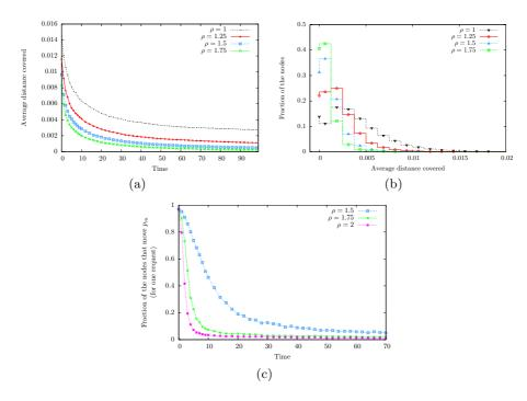
**Fig. 5.** Evaluation of Grasp in a 2D toric ROI: (a) average distance covered per node (relatively to R) as a function of time ( $\lambda=1$ ); (b) load distribution in the systems with respect to the average distance to be covered by a node to deliver a message (relatively to R); and (c) the probability that Grasp uses mobility to deliver a message as a function of time ( $\lambda=10$ )
