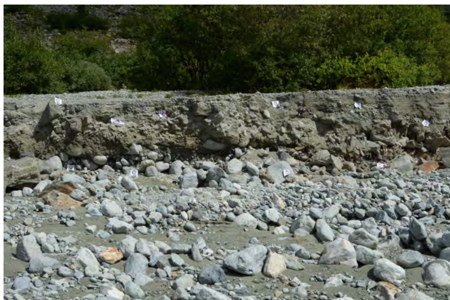
Figure 4.2 – Riverbank of the Borgne d’Arolla, Valais, Switzerland. 10 targets printed on regular paper are disposed along it for referencing purposes.
