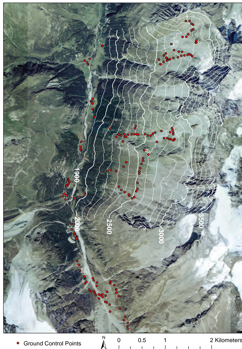
Figure 7.2 – Ground Control Point distribution in the Arolla Valley, Switzerland (Contour line spacing: 100 m, Orthophoto: Swisstopo 2005).
