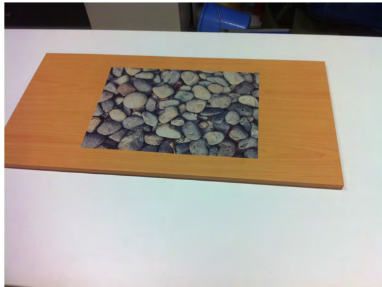
Figure 4.7 – Set up for the experiment: high quality print pasted on a wooded plank to be as flat as possible.
