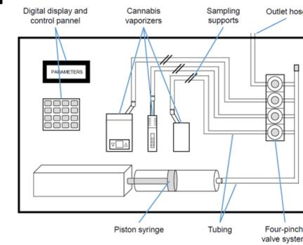
Fig1. Schema of the smoking machine
