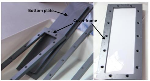
**Figure 3. Large-surface DGT device for environmental Pu speciation measurements.** Parts of the DGT device — the bottom plate and the cover frame — depicted on the left, the assembly with crew holes on the right.
