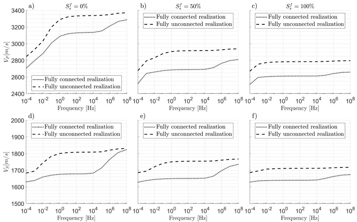
Figure 3: (a, b, c) P- and (d, e, f) S-wave velocities as functions of frequency for a single realization of connected (dotted lines) and unconnected (dashed lines) fracture networks. Steam saturation of the fractures  $S_s^f$  is (a, d) 0%, (b, e) 50% and (c, f) 100%.
