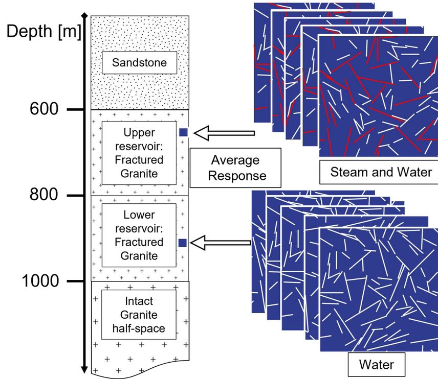
Figure 6: Schematic representation of the geothermal reservoir model employed in the analysis. The sandstone and intact granitic layers are considered to be homogeneous, while the granitic reservoir is characterized as a fractured formation with the fractures being saturated with either water and steam (upper part of the reservoir) and only water (lower part of the reservoir).
