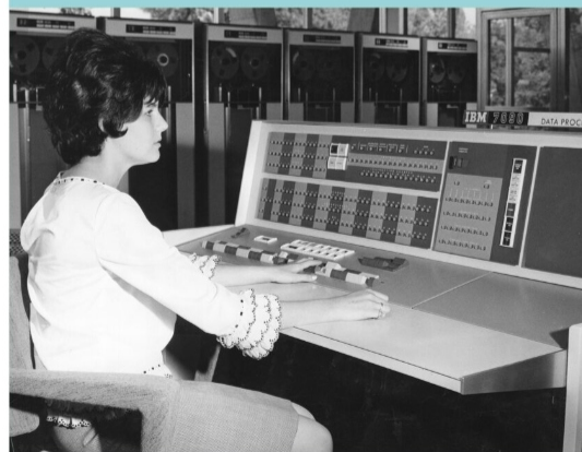
The console of the IBM 7090, the computer used by Dearing (1962) for one of the first collation programs. Courtesy of International Business Machines Corporation, © (1961) International Business Machines Corporation.
