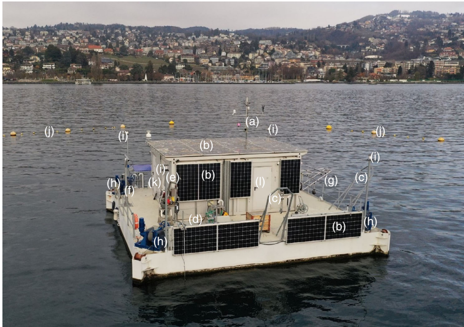
FIGURE 1 Side view of LéXPLORE from the south with the town of Pully in the background. The image shows the sheltered laboratory and exterior meteorological instruments (a), solar panels (b), on roof and towards south, two A-frames (c), the outdoor moonpool (d) with electrical winch (e), support frame for lifting loads (f), and the structure maintaining a thermistor chain (g). Blue anchor winches with cables for positioning rest at all four corners (h) and are mounted with navigation lights (i). The two doors access the toilet (k) and the laboratory (l). Battery banks and diesel-generator rest inside the pontoon-hull. The yellow buoys delineate the safety perimeter (j) for instrument protection. Reprinted with permission from Florian Bentlee, Stuttgart, Germany
