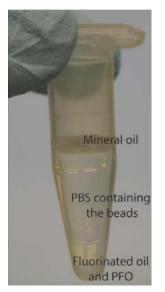
Figure 3. Three phases after breaking the emulsion
