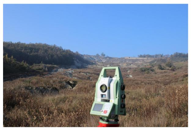
Figure 36. The Leica Nova MS50 used for Roncovetro landslide traditional monitoring.
