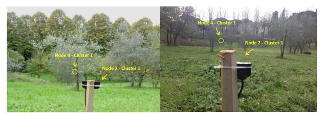
Figure 15. Line of sight between antennas 2-4 of Arcetri Cluster 1 before and after changes (respectively on the left and on the right).
