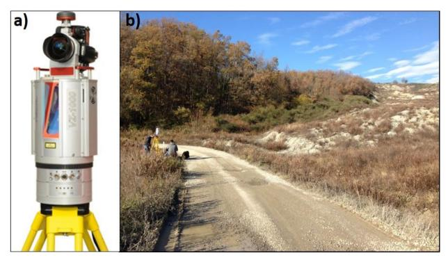
Figure 69. Laser scanner survey. a) the employed RIEGL VZ-1000 laser scanner; b) picture taken during the survey (scan position 1 of Figure 68).
