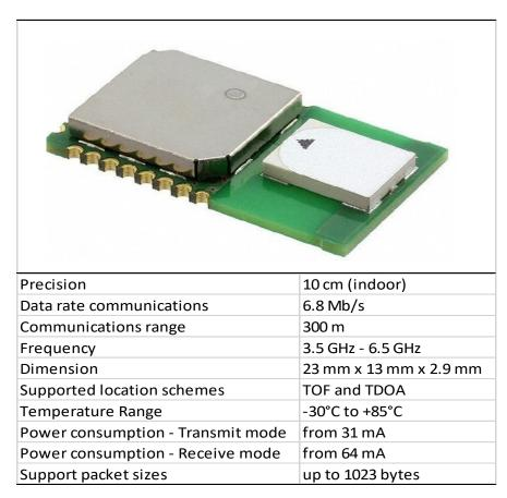
Figure 10. Detail of the Ultra-Wide Band module used in the Wi-GIM system, the Decawave Sensor DWM1000. For more detail, please visit the Decawave website (https://www.decawave.com/product/dwm1000-module).
