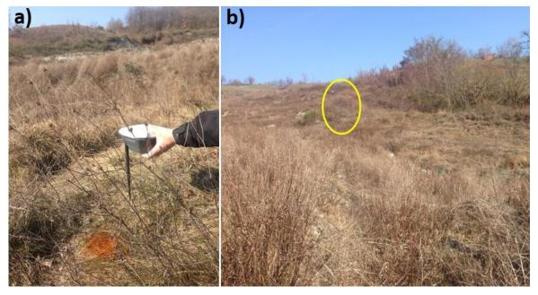
Figure 76. Wi-GIM installation after the implementation of WiSIO. a) Emlid Reach RS+ GPS point finder function used to localise the Points detected by the algorithm; b) installation of the new Cluster 1 Node 8 (highlighted with a yellow circle).
