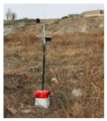
Figure 37. Prism targets installation on the same pole of the Wi-GIM antennas.
