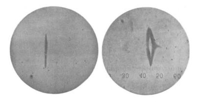
Figure 1: Pattern created by a ray of silver atomes in the original Stern-Gerlach experiment: left without, right with magnetic field.
