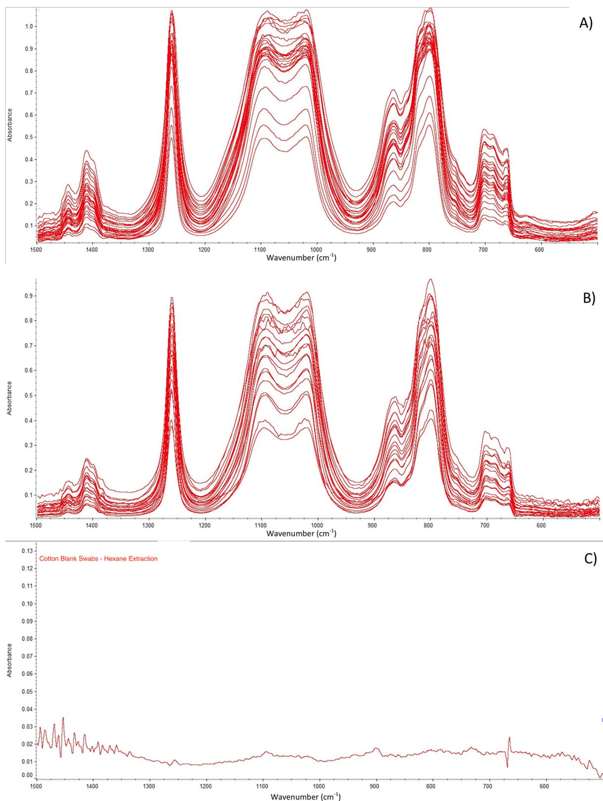
**Fig. 3.** Illustration of the spectra obtained A) after hexane extraction, B) after DNA followed by Hexane extraction, C) blank cotton swab.
