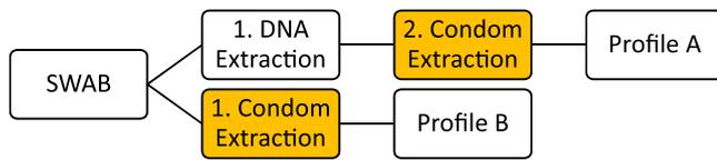
Fig. 1. Illustration of the extraction sequence.
