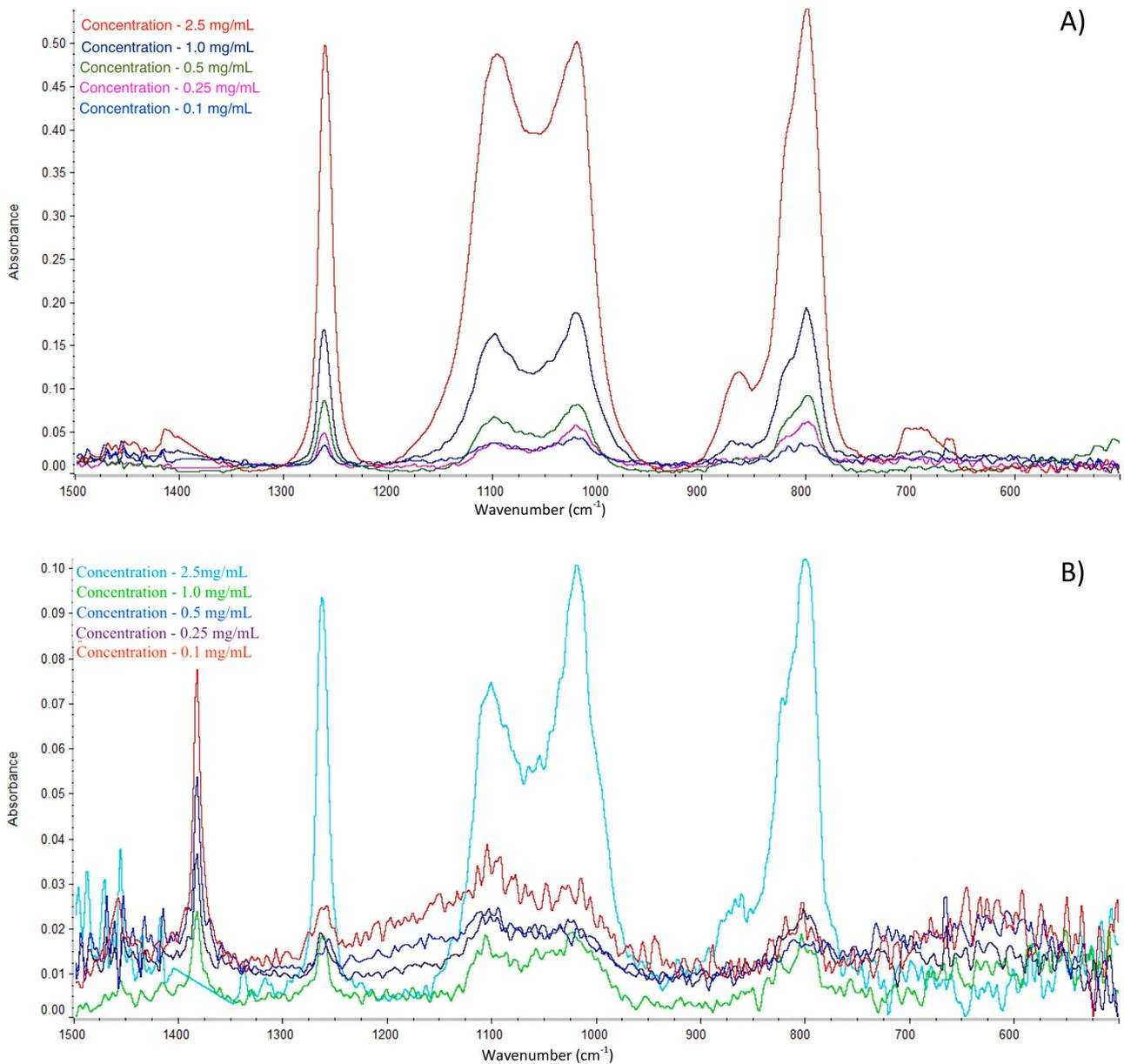
**Fig. 5.** : Illustration of the decrease of the concentration A) after direct hexane extraction, B) after DNA followed by hexane extraction.
