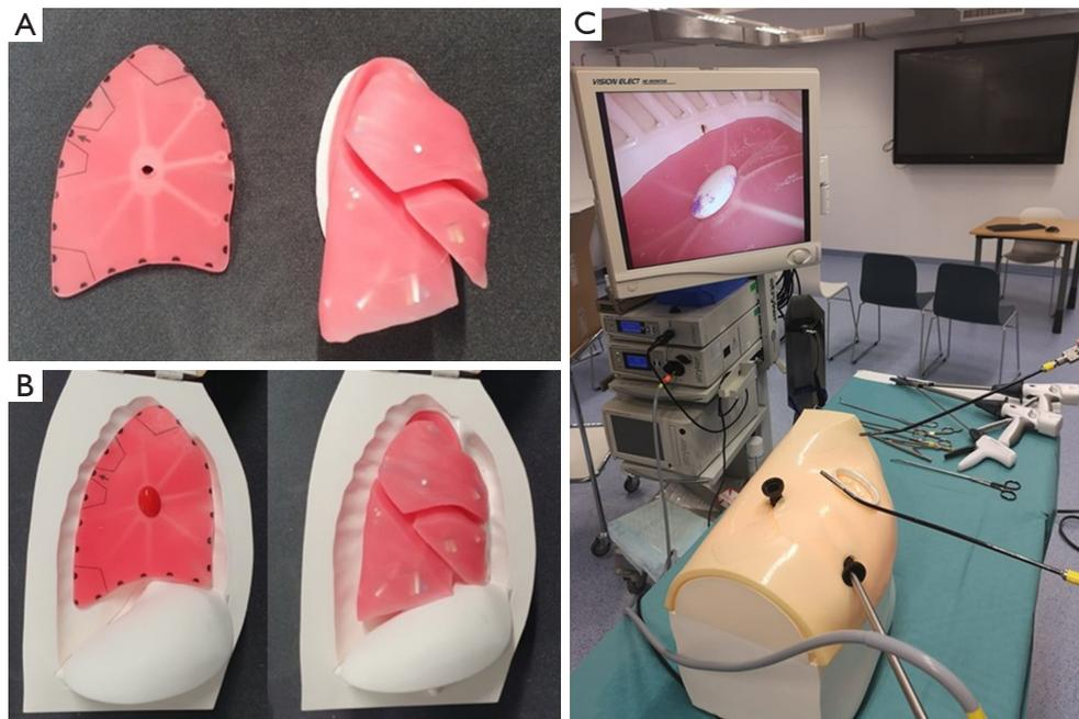
**Figure 2** The Johnson & Johnson Ethicon Stupnik® VATS simulator. (A) 2D and 3D lung model inserts. (B) Inserts placed into the mannequin. (C) Final setup with thoracoscopy tower including monitor, light source, optic and thoroscopic instruments. VATS, video-assisted thoracoscopic surgery; 2D, two dimensional; 3D, three dimensional.
