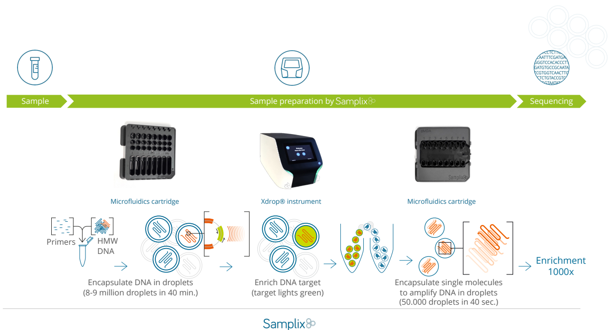
Figure 2.1.2: Xdrop enrichment workflow (As provided by Samplix)
