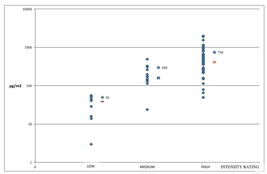
Figure 3 Available PCB air concentrations by exposure group rating: high, medium, and low PCB exposures. Group GMs (low ( +), medium ( ), high ( )) and their given exposure ratings ( ) with concentration value) are also indicated.
