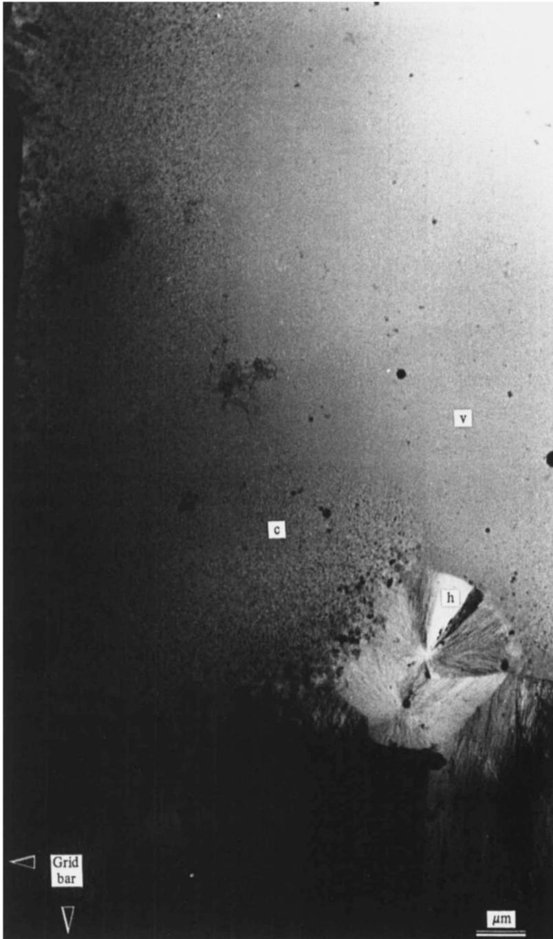
Fig. 48. Thin layer of nearly pure water in which hexagonal (h) and cubic (c) ice coexist with vitreous water (v). The thinnest region of the film is vitreous whereas the thicker regions, close to the grid bars, are crystallized.
