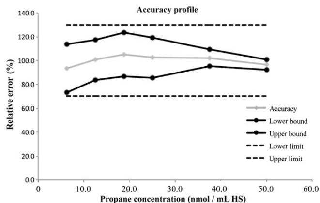
**Figure 3.** Accuracy profile of propane gas according to the GTFCh protocol using a simple linear regression model within a range of 6.30–50 nmol/mL of HS vial (continuous light gray line: trueness, black dotted lines: acceptance limits set at  $\pm 30\%$ , black gray lines: lower and upper accuracy limits in relative values).
