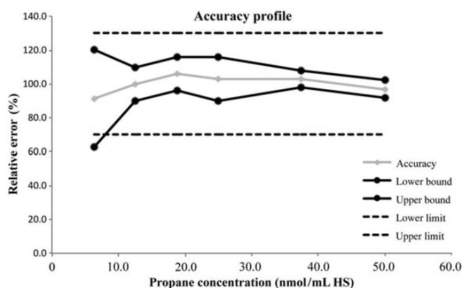
**Figure 2.** Accuracy profile of propane gas according to the SFSTP protocol using a simple linear regression model within a range of 6.30–50 nmol/mL of HS vial (continuous light gray line: trueness, black dotted lines: acceptance limits set at  $\pm 30\%$ , black lines: lower and upper accuracy limits in relative values).
