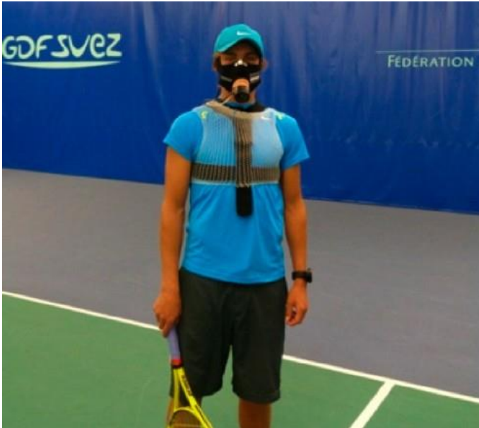
Picture 1 – Player's equipment (gas analysis system) during TEST.
