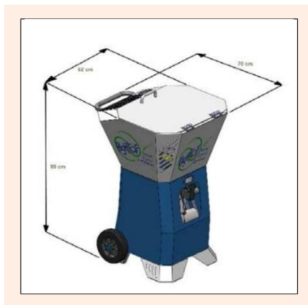
Figure 1. Dimensions of the 'Hightof' ball machine.
