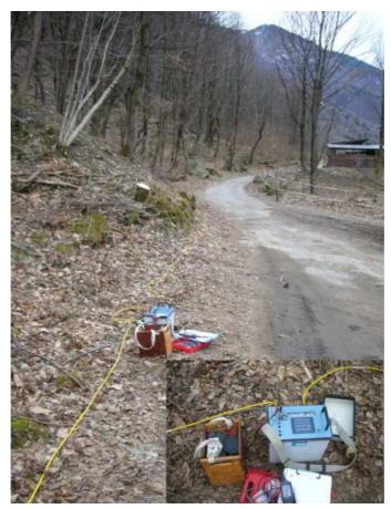
Figure 3.5 - IRIS SYSCAL PRO used for the geophysical surveys. The big picture shows the equipment with the spread-out multicore cable, while the small insert picture shows in more detail the used instrument.
