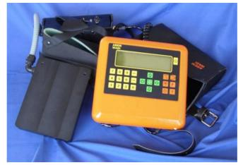
Figure 3.13 - The ABEM® WADI VLF-EM instrument used in this research project.
