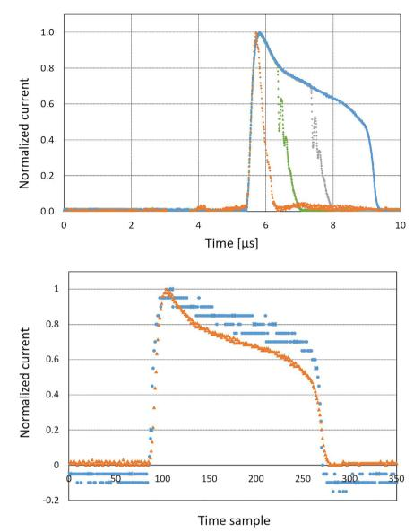
**FIGURE 3** Comparison of the normalized raw signal from the initial monitor system (blue circles) and the newly mounted beam current transformer (BCT) (orange triangles) for same ultrahigh dose rate (UHDR) pulse
