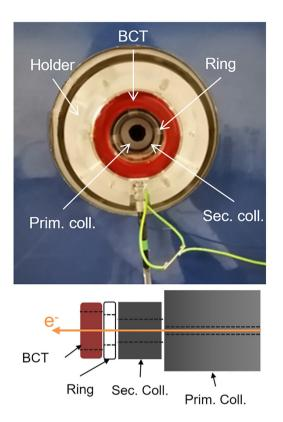
**FIGURE 1** Picture of the holder at the exit of the linac (top) and scheme of the complete setup showing the beam current transformer (BCT), a PMMA ring, and both secondary and primary carbon collimators (bottom). The physical apertures of these devices were 55, 50, 40, and 12.4 mm, respectively. The inner diameters of the manufactured elements were chosen based on lateral dose profiles acquired at the same position
