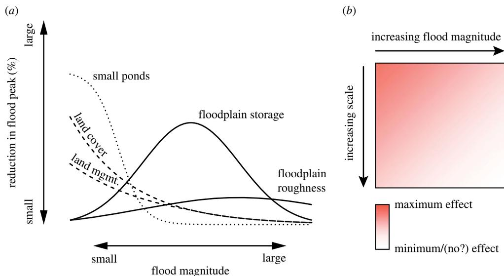
**Figure 3.** Schematic diagram showing relative effects of catchment-scale interventions on flood peaks. (a) Effect of different types of intervention on flood peak reduction  $[E_{xp\_op}]$ ; (b) combined effect of CBFM interventions with flood magnitude and catchment scale  $[E_{xp\_op}]$ . We note that the effects achievable in practice will depend on the details of the particular intervention and the context in which it is deployed.
