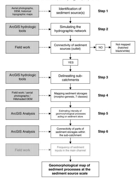
Fig. 1. Flow chart illustrating the procedure used in the presented mapping method for small alpine catchments.
