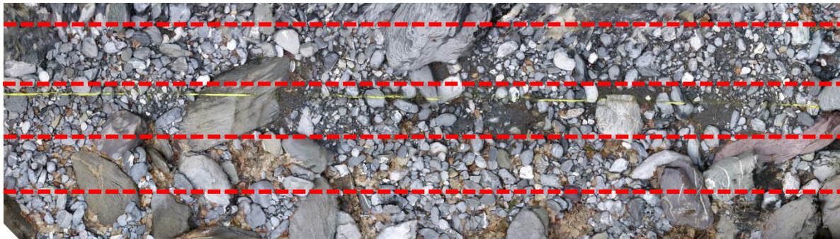
Figure III-S.3. Lines through the emerged areas of the streambed, based on which the representative grain-size class D_{50} and D_{84} were determined.
