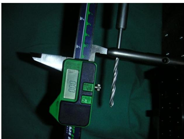
**Figure 4** Calibration of the testing apparatus in the neutral position without external forces being applied to the nail.
