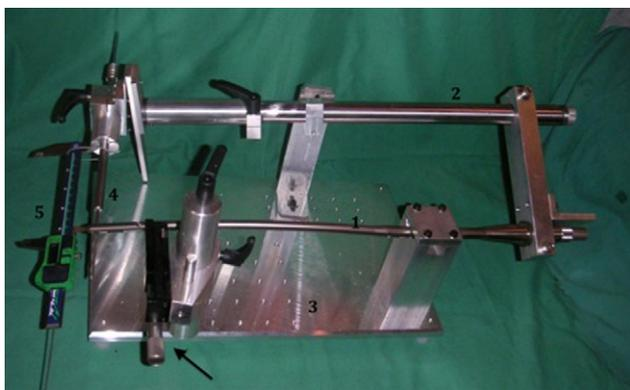
**Figure 3** Overview of the testing apparatus. An intramedullary nail (1) with a proximally mounted aiming arm (2) was solidly fixed on a bench (3). After calibration of the system, the nail was progressively bended by dressing the clamp (arrow) until the passage of the drill bit (4) through the locking hole of the nail was not possible. The amount of nail bending was indicated on the calliper (5).
