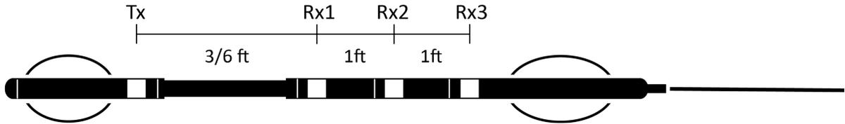
**Figure 1.** Schematic illustration of the used sonic logging tool with one transmitter (Tx) and three receivers (Rx1, Rx2, Rx3). The offset to the source of the first receiver is 3 and 6 ft for the short and long tool configurations, respectively.
