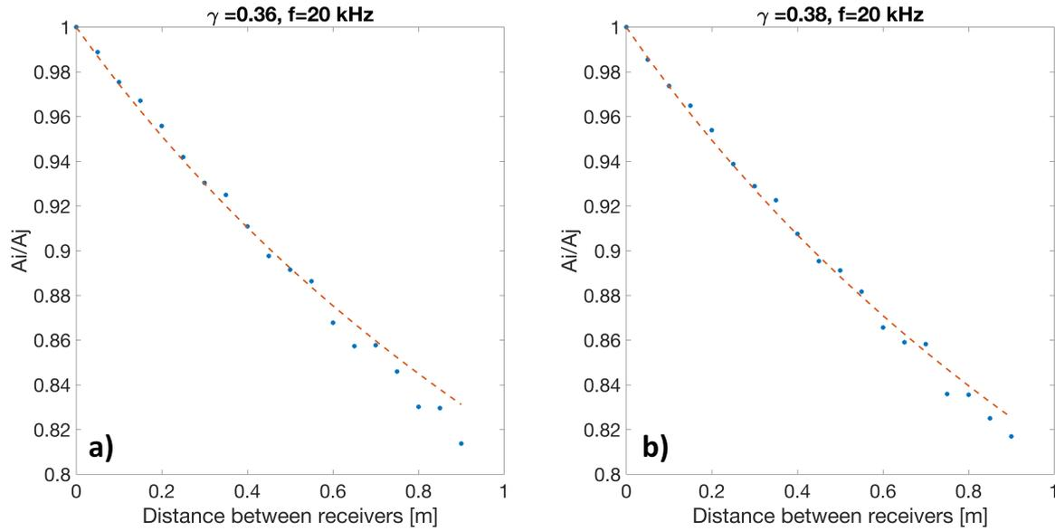
**Figure 4.** Geometrical spreading exponent  $\gamma$  computed from spectral ratios at  $f=20$  kHz obtained using numerical simulations of wave propagation (dots) for cases 1 (a) and 2 (b) in Table 3. The dashed curve shows the spectral ratios obtained with Eq. 6 using the  $\gamma$ -value indicated in plot.
