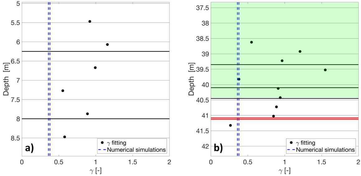
**Figure 5.** Geometrical spreading exponent  $\gamma$  computed for the upper (a), and lower (b) sections. The depth of the dots indicates the mid point of the interval between two corresponding receivers. The blue dashed lines show the range of values of  $\gamma$  computed using the numerical borehole model. Regions colored in green correspond to shear zones. Black lines and red layers correspond to fractures and dykes, respectively.
