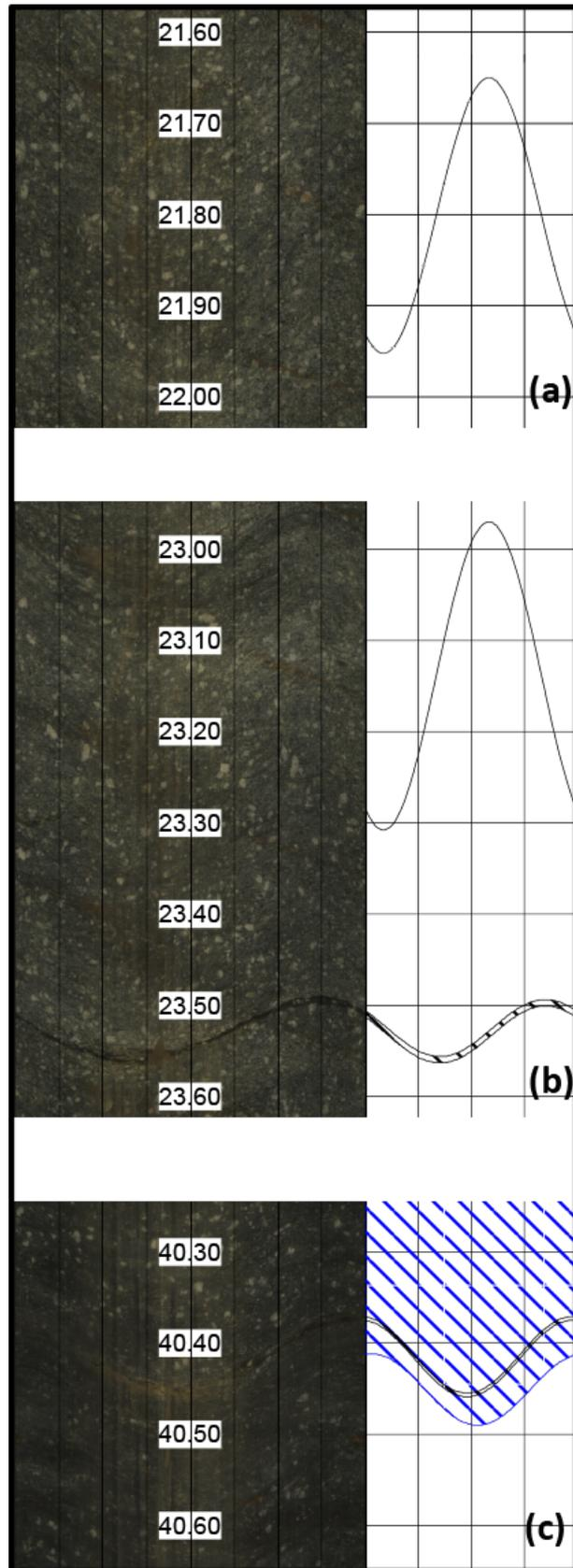
**Figure 10.** Televiwer image and its interpretation for the fractures in the central and lower sections given in Table 4. Shear zones are identified with diagonal blue lines.
