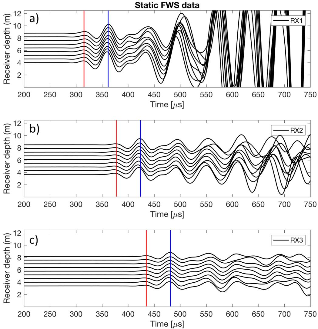
**Figure 2.** Static FWS data recorded in the upper section of the borehole for receivers (a) Rx1, (b) Rx2, and (c) Rx3. The offset to the source of the first receiver corresponds to the short tool configuration. The red and blue vertical lines illustrate the central time of the time windows employed to isolate one and two cycles of the first P-wave arrival, respectively.
