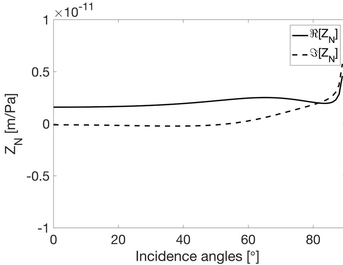
**Figure 11.** Real and imaginary components of the fracture compliance computed using Eq. 13 and considering the P-wave transmission coefficient at different incidence angles.
