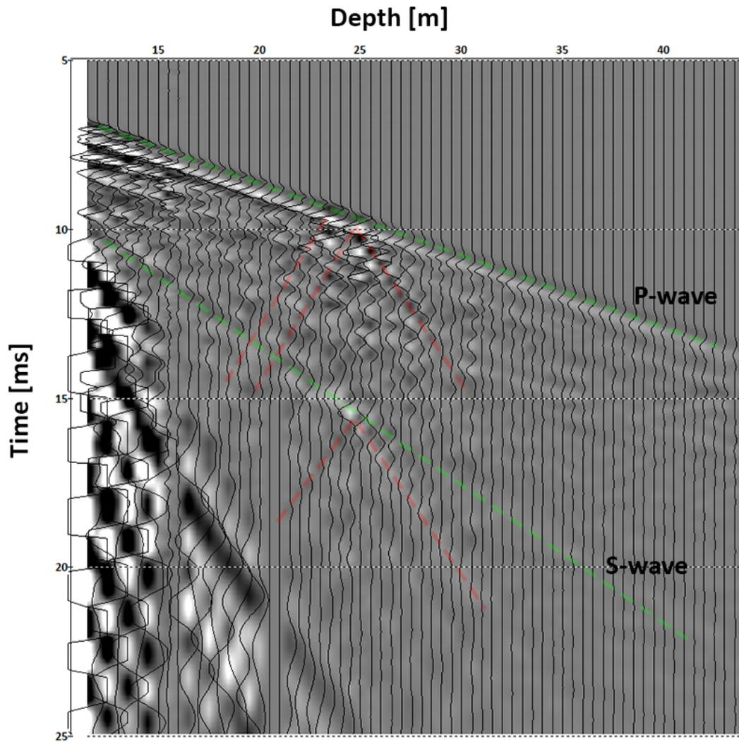
**Figure 12.** Zero-offset hydrophone VSP data collected with sensors located at depths ranging from 11.5 to 44 m along the INJ2 borehole. The green lines denote the arrivals of the P- and S-waves propagating along the borehole wall. Red lines correspond to the arrivals of tube wave generated at the fractures.
