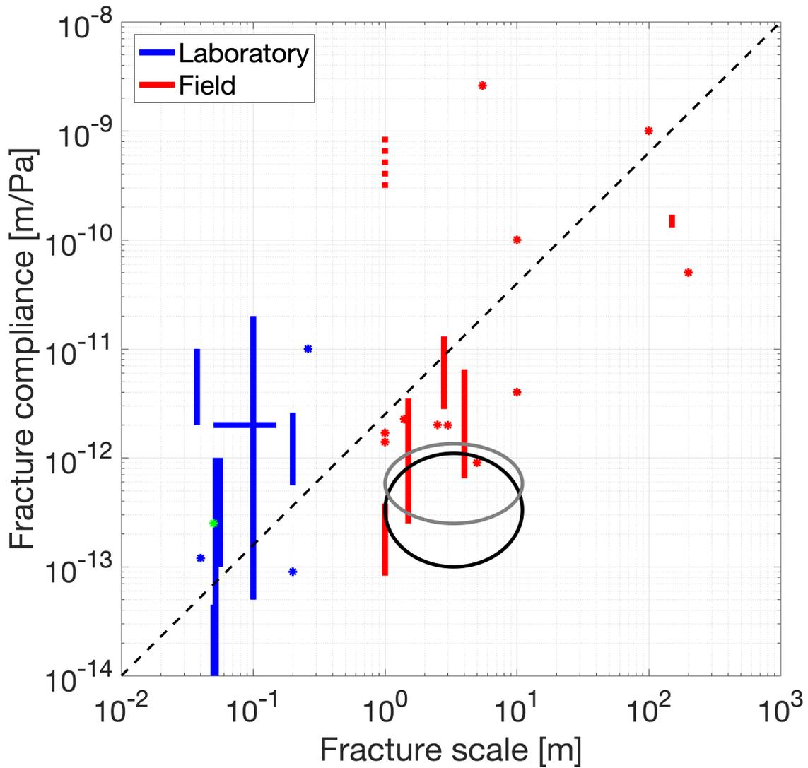
**Figure 13.** Static (blue) and dynamic (red) fracture compliance values as function of fracture size compiled from the literature. The black and grey ellipses indicate the range of the real component and absolute value of the compliances reported in this work, respectively. The green dot corresponds to the compliance estimated from the laboratory measurements on synthetic samples by *Rathore et al.* [1995].
