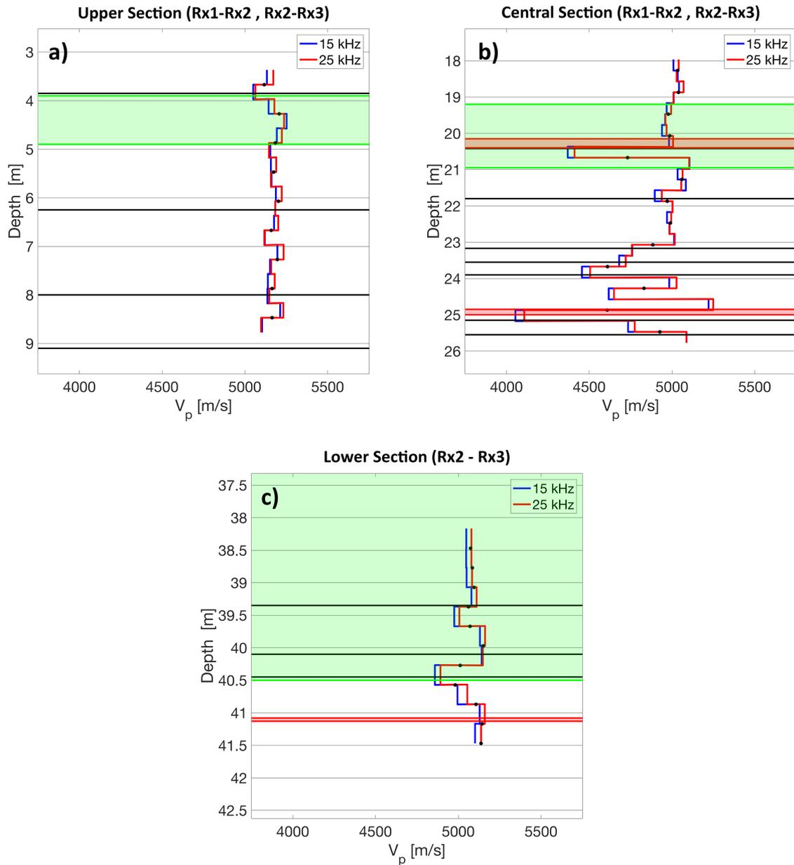
**Figure 3.** P-wave velocity computed for the nominal source frequencies 15 kHz and 25 kHz in the upper (a), central (b), and lower (c) sections of the borehole. Regions colored in green correspond to shear zones. Black lines and red layers correspond to fractures and dykes identified in televiewer images, respectively. Dots illustrate the interval velocity between first and third receivers at the corresponding mid-point.
