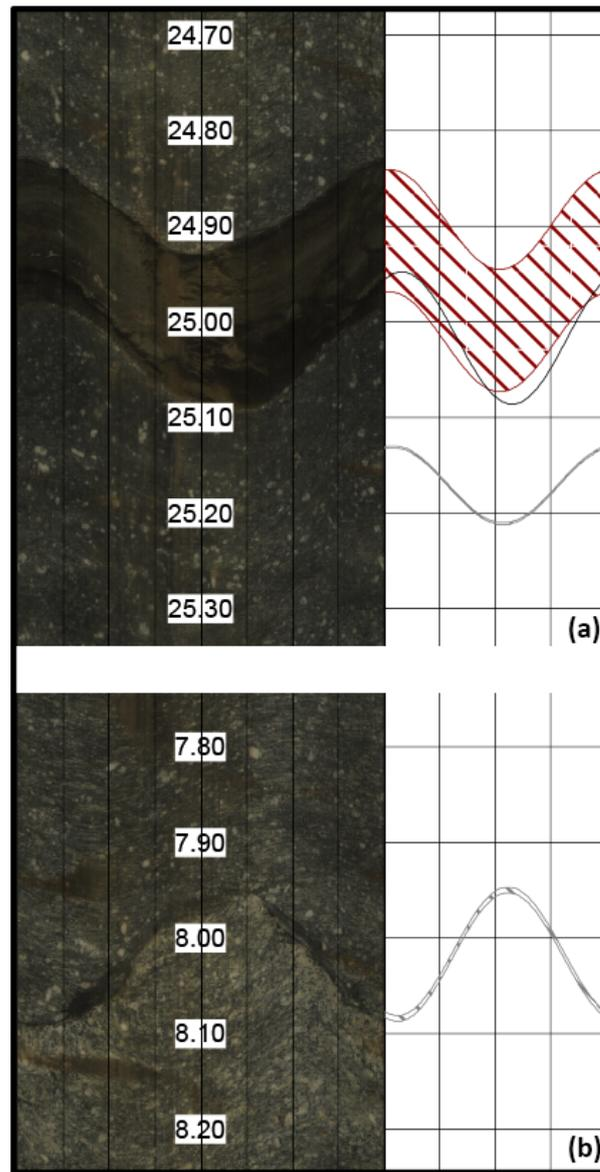
**Figure 9.** Televiewer images [Krietsch *et al.*, 2018] of (a) a dyke (red layer) and (a, b) fractures (dark lines) in different sections of the borehole.
