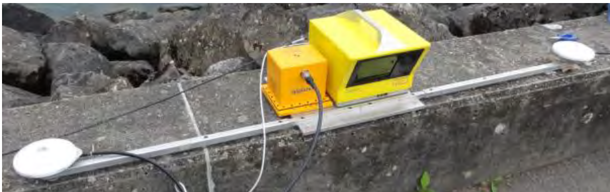
Figure 3.5: Setup of the Optech IlrisER TLS (yellow box with control screen) close to the Applanix IMU (orange box) and of the 2 GNSS antennas fixed at each side of the central plate on rigid arms.
