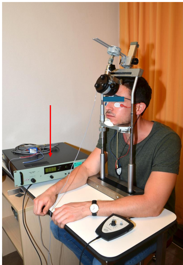
Fig. 2. Frontal stimulation. Modified slit lamp holding the bone vibrator and allowing a three-dimensional adjustment of the position of the bone vibrator on the patient’s forehead. The small digital display on the Brüel and Kjaer amplifier type 2718 (red arrow) showed the electrical current delivered by the device according to the pressure applied, allowing the optimal pressure on the forehead to be adjusted.
