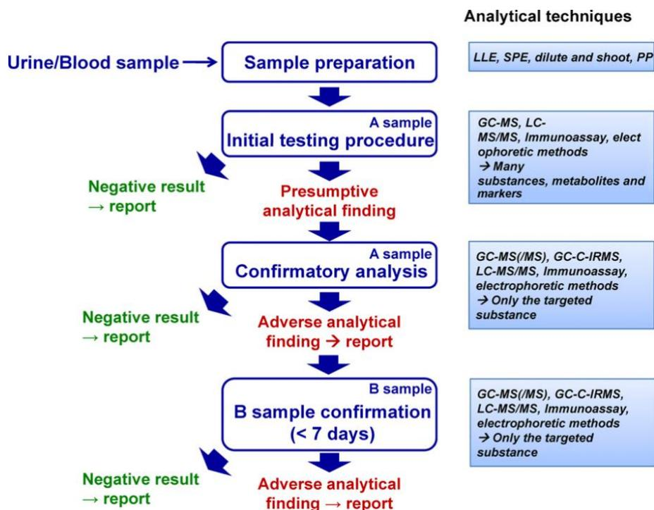
Figure 2. Workflow for anti-doping analyses [15]
