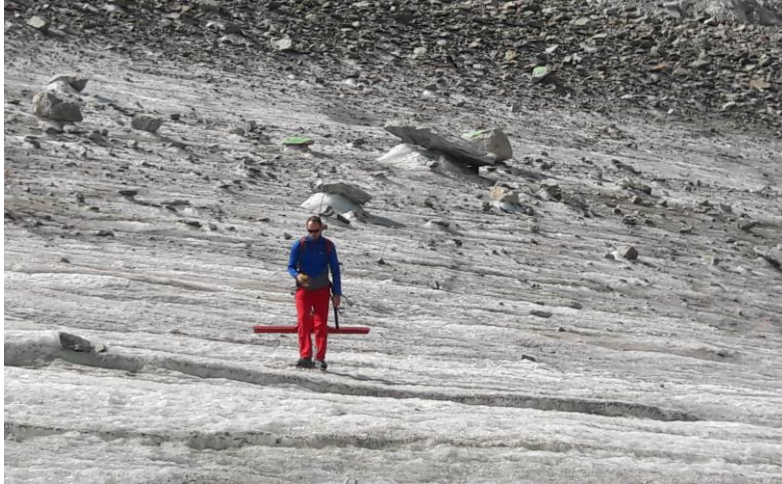
Figure I-3: GPR survey at Glacier d’Otemma in summer 2018, using a single Radarteam® transmitter-receiver antenna mounted on a backpack, and a dGPS rover antenna for positioning and navigation. Photo: Pascal Egli.
