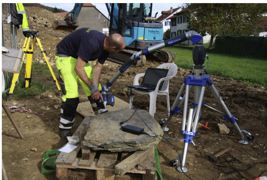
Fig. 3. The FARO ScanArm® Quantum V3 used to scan one of the smaller stones of the dolmen.
