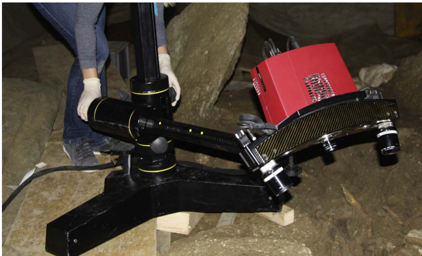
Fig. 9. Difficult positioning of the GOM ATOS III fixed on an about 70–80 kg steel stand with outrigger, as it has to be stable and leveled.
