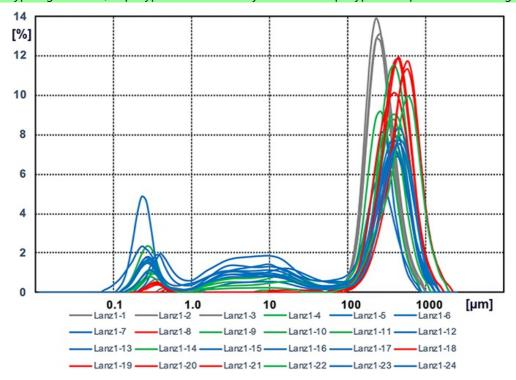
Figure 4. (colour online) CaCO<sub>3</sub> content and Volume-% of the three generalized grain size class 1 (0.1–1.0  $\mu$ m), class 2 (1–60  $\mu$ m) and class 3 (60–2500  $\mu$ m). The data are listed in Table 2. Banks 1–3 refer to Figure 2.
