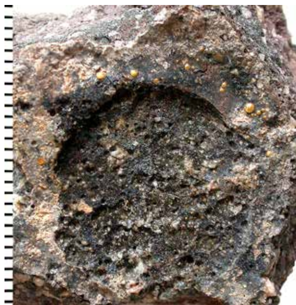
Fig. 3. Methone: detailed view of pellet imprint and gold globules in the vitrified layer of a melting plate (photo S. Verdán)
