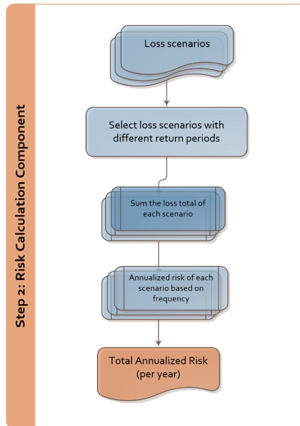
Figure 4.6. Workflow of the risk calculation component. The loss scenarios with different return periods are combined to obtain the total annualized risk (per year) based on the staircase approach.
