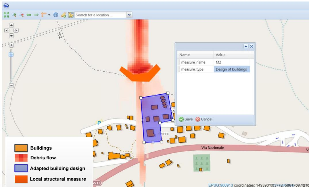
Figure 5.11. An example proposition of risk reduction measures by an expert user through a sketching tool of the prototype platform.
