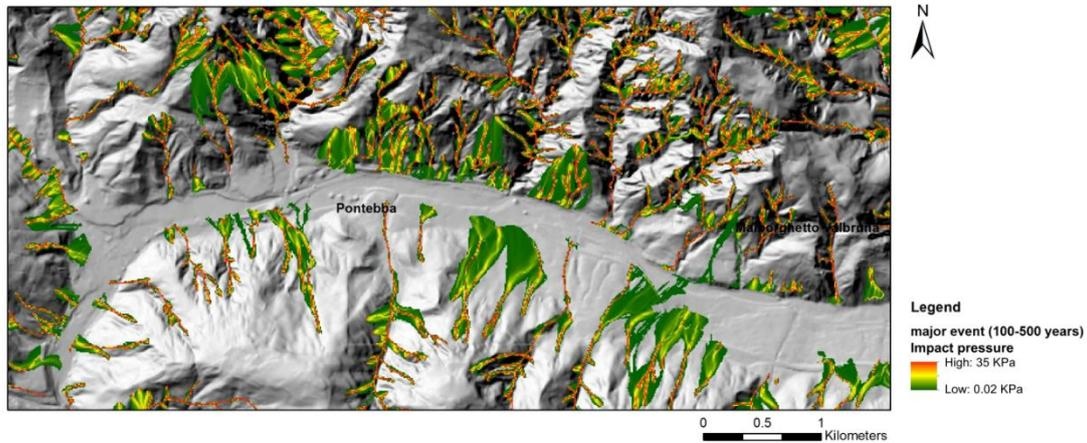
Figure 4.10. Debris flow (maximum intensity) of major event with return periods of 100–500 years (Hussin et al., 2014b).
