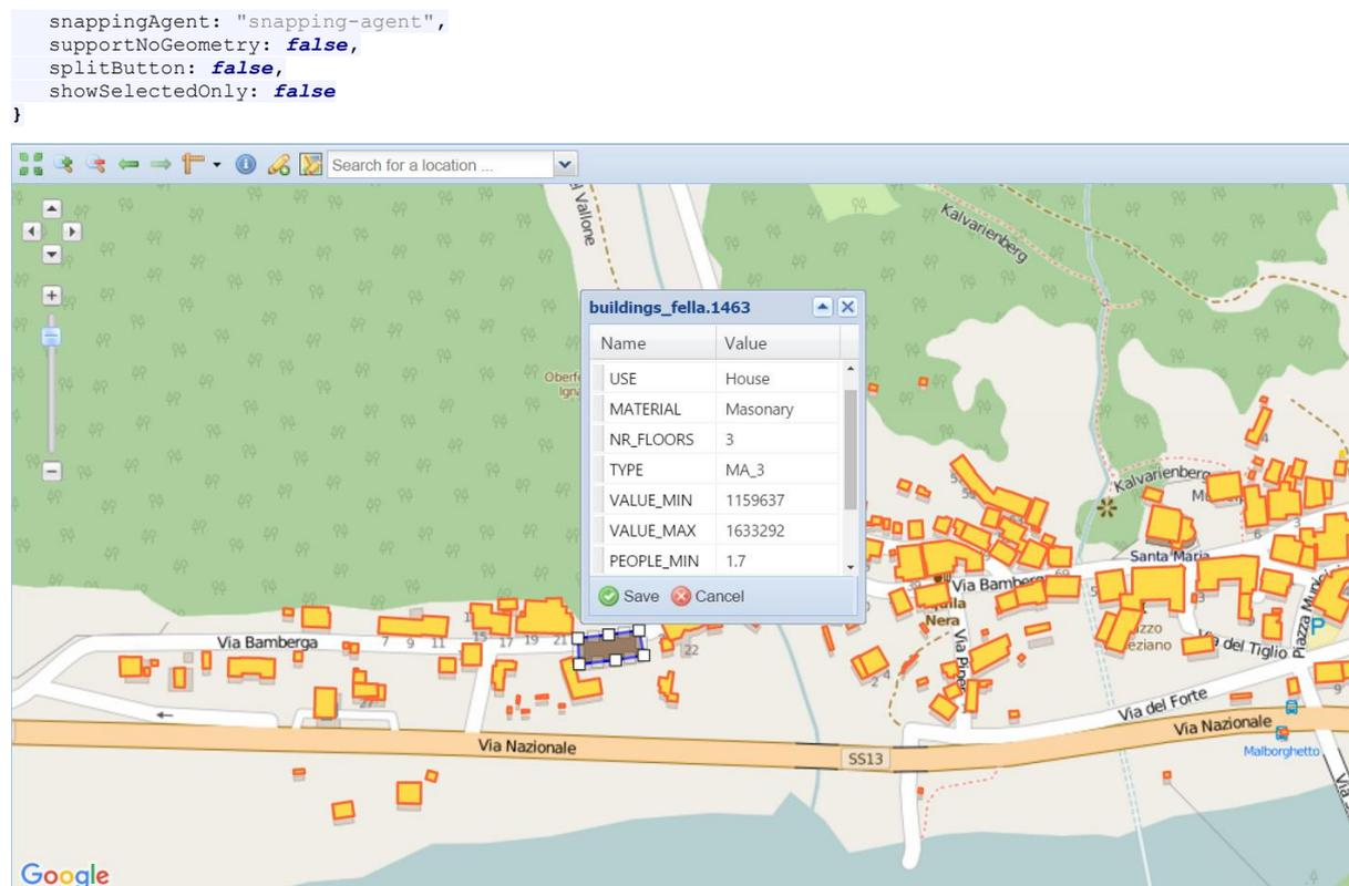
Figure 2. The user interface for editing of features in the vector layer (using FeatureEditor plugin).
