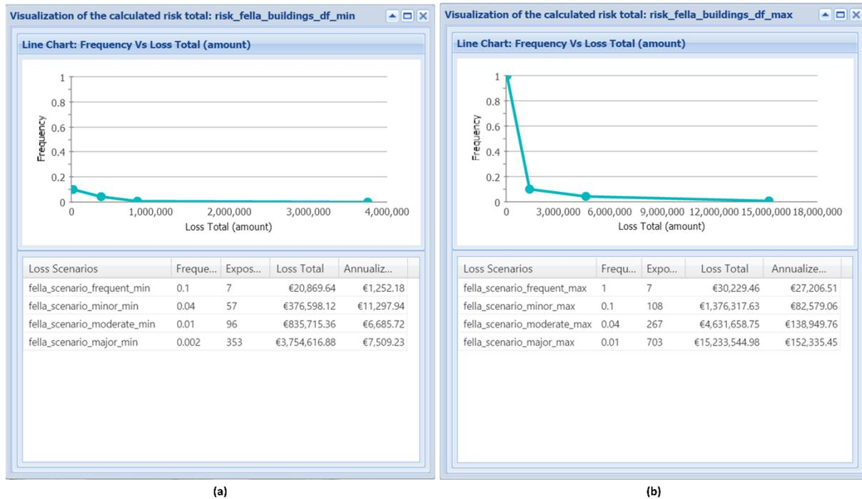
Figure 4.14. (a) Visualization of the debris flow risk curve (minimum). (b) Visualization of the debris flow risk curve (maximum).
