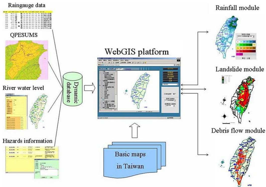
Figure 3.2. Components of the web-GIS platform for slope land hazard warning (Source: Yu et al., 2007).
