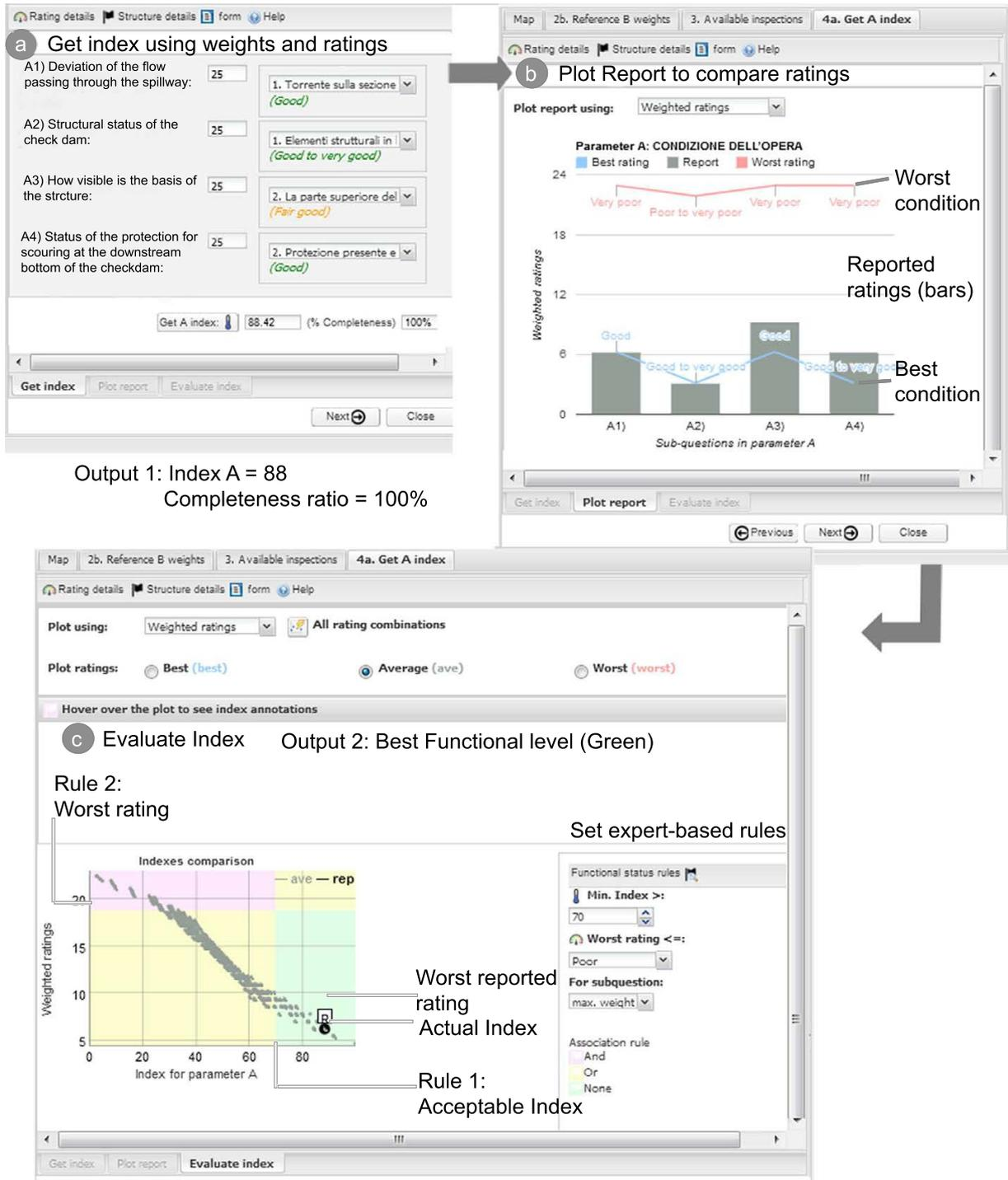
Figure 9: Outputs from the evaluation module: a) Index and a completeness ratio indicating the reported ratings. b) Report plot to compare ratings with reference conditions. c) Functional category of the parameter according to expert-based rules
