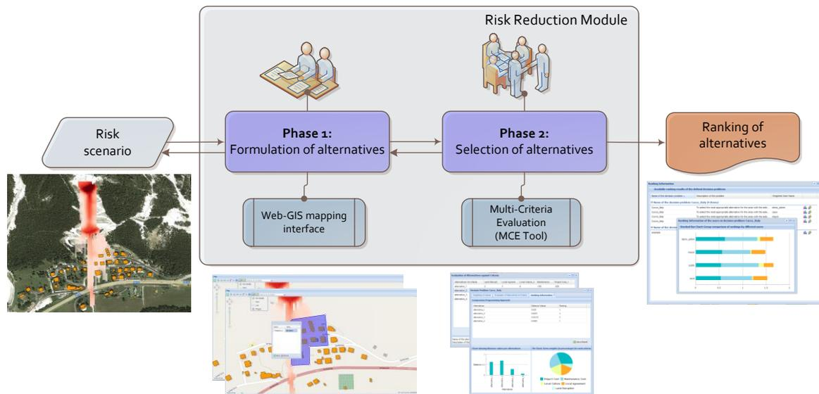
Figure 5.2. A collaborative two-phase framework of the risk reduction module of the prototype platform. Risk scenarios are obtained from the risk analysis module (see Figure 4.1 and Chapter 4). Different types of users exist and the detailed interaction of who is involved in which phases is explained in Table 5.1.
