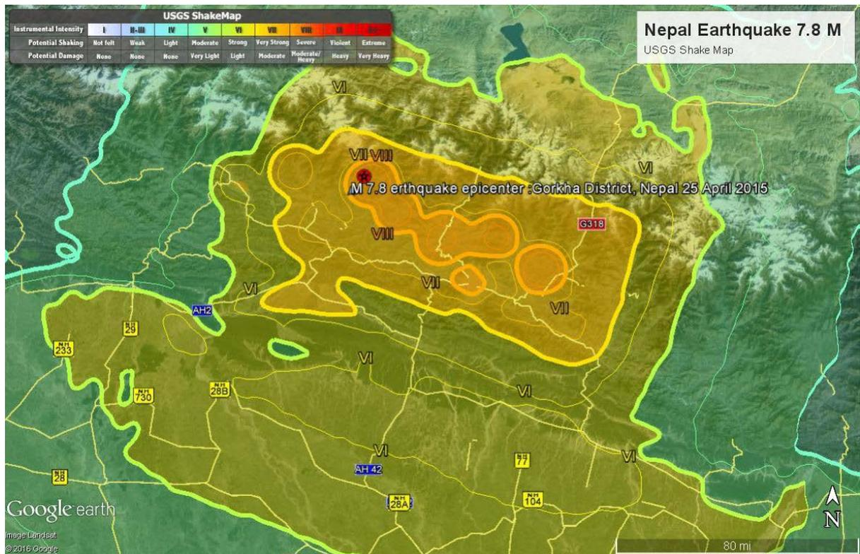
Figure 5 Shaking intensity map of Earthquake 7.8 M (Source of Data: [17])
