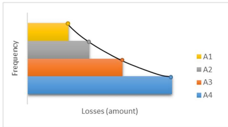
Figure 4.3. An example of risk curve in the form of staircase. A1–A4 represents the area derived from the loss calculation for four return periods. Each A1–A4 contributes to the risk total ( $R$ ) of the considered hazard event (e.g. debris flows).
