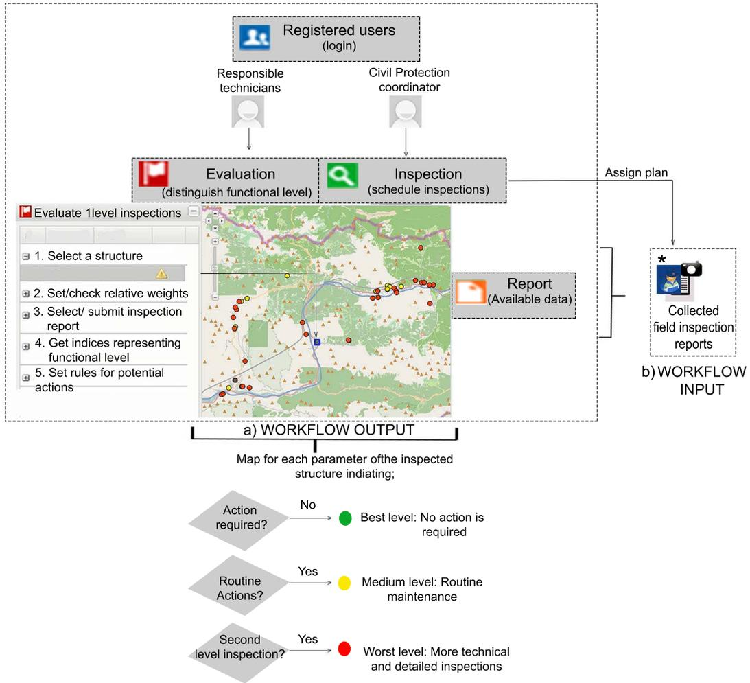
Figure 1: Workflow describing the input and output information for the decision support framework. \*Volunteer icon (Civil Protection of FVG region, Italy)
