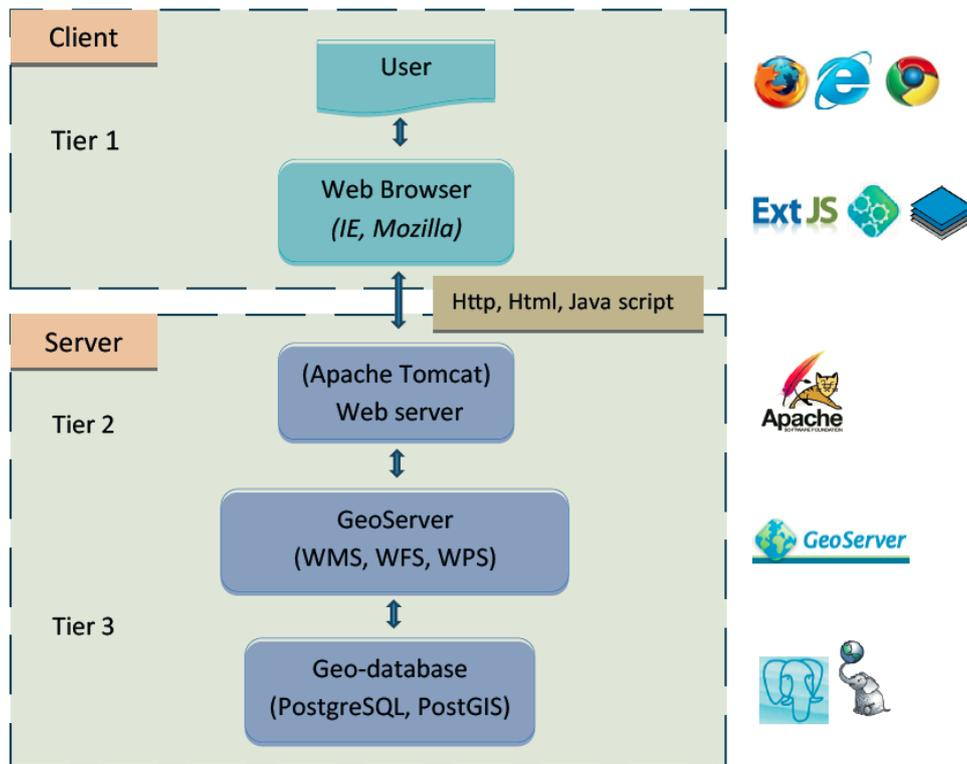
Figure 3.6. Schema of the three-tiered client-server architecture for the web-GIS applications.
