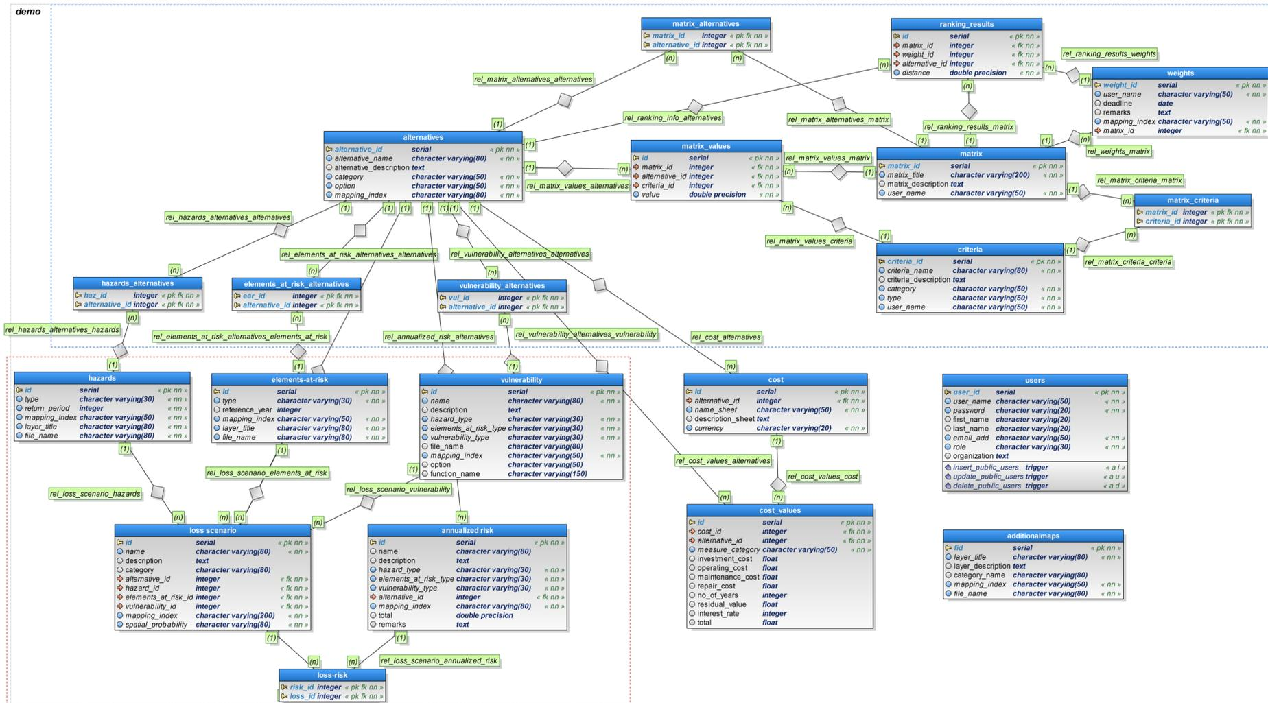
Figure 2. Global data model of the schema (in this case, demo). The lower (dotted line in pink colour) part of the model represents the background data structure of the data management and risk analysis modules (see 4.7 of Chapter 4), while the upper (dotted line in blue colour) part represents the alternative management and decision analysis modules (see 5.5.2 of Chapter 5).
