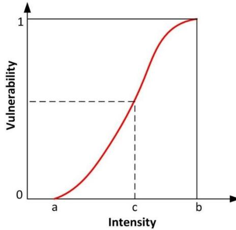
Figure 4.2. An example illustration of a generic vulnerability curve using a Cumulative Distribution Function (CDF). The input parameters  $a$ ,  $b$  and  $c$  are obtained from the user to generate the vulnerability curve with or without class (type) information for a certain category of elements-at-risk.
