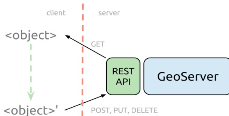
Figure 3.9. REST interface of GeoServer (Source: Boundless, 2012).
