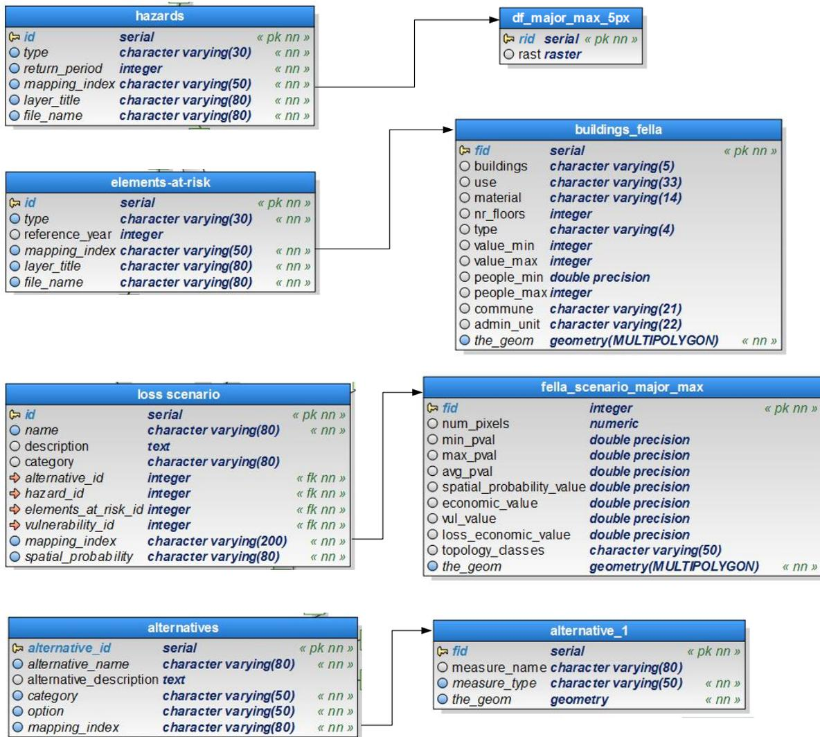
Figure 3. Illustration of relationships with dynamically created spatial tables in the data model (schema). The 'mapping\_index' attributes of the main non-spatial tables (on the left) store names of the spatial tables (on the right) to create a link between them. For example, 'mapping\_index' attribute of the 'alternatives' table stores the value 'alternative\_1' to create a connection with the newly created alternative table.
