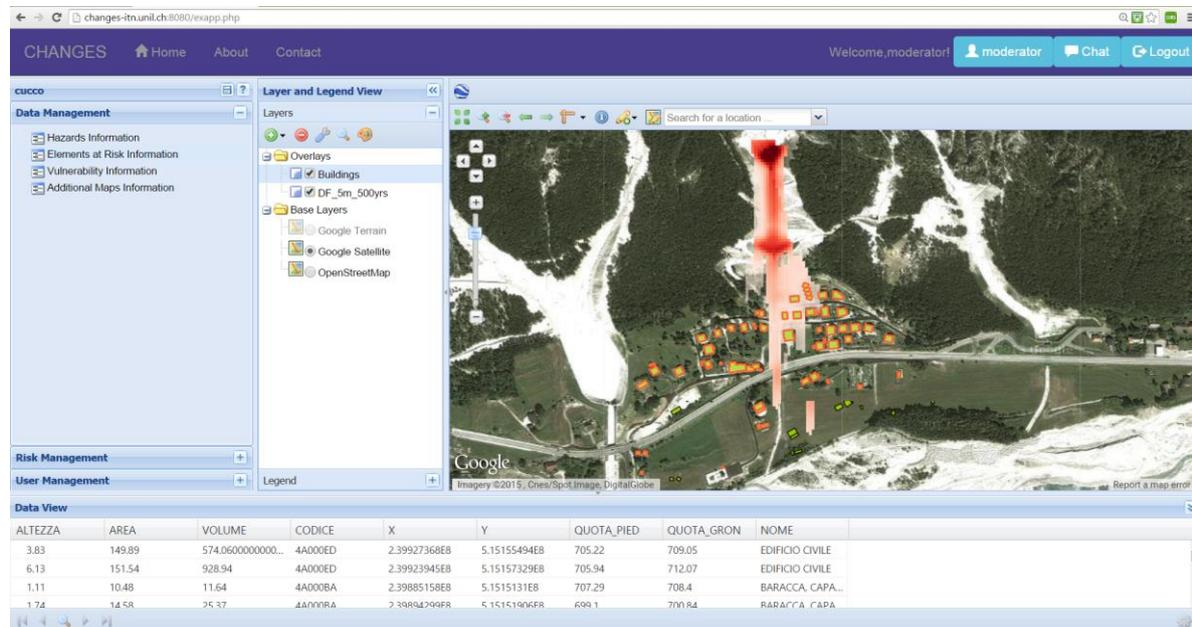
Figure 3. Overlay of debris flow and building maps of Cucco village.
