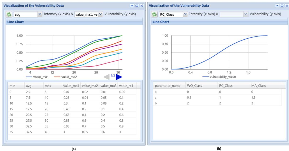
Figure 4.12. (a) Visualization of the vulnerability curves generated using data ranges. The curves are drawn based on the average intensity values for different building material types such as masonry 1 floor, reinforced concrete 1 floor, etc. (b) Visualization of the vulnerability curve generated using the CDF. The curve is drawn based on Eq. (4.2) for the building material type (e.g. reinforced concrete). The input parameter values a, b and c are given by the user.
