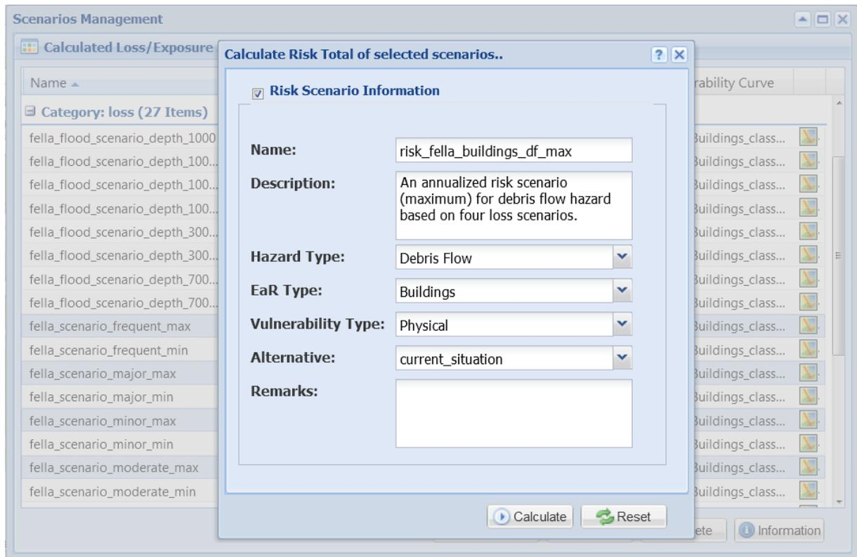
Figure S7. The interface of the risk component illustrating the selection of loss scenarios for calculation of an annualized risk scenario. At least three or more loss scenarios with different return periods are required, and the user can enter related information such as name, description, hazard, elements-at-risk and vulnerability type of the calculated risk scenario.
