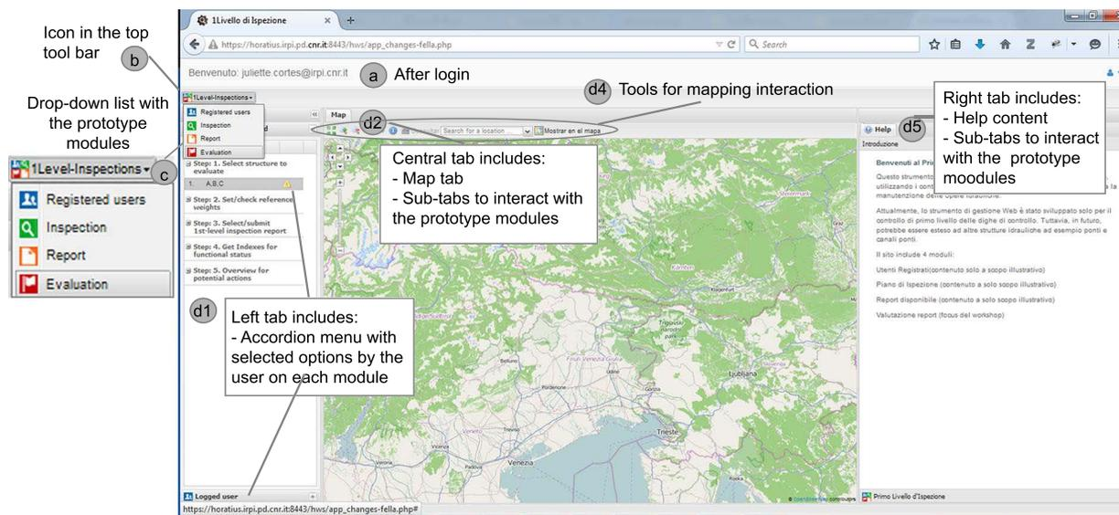
Figure 5: Web-GIS platform interface indicating a) Registered user; b) Decision support prototype; c) Drop down list to access the modules; d) Content in the left, central and right tab-panel. The central tab-panel includes the tools for mapping interaction
