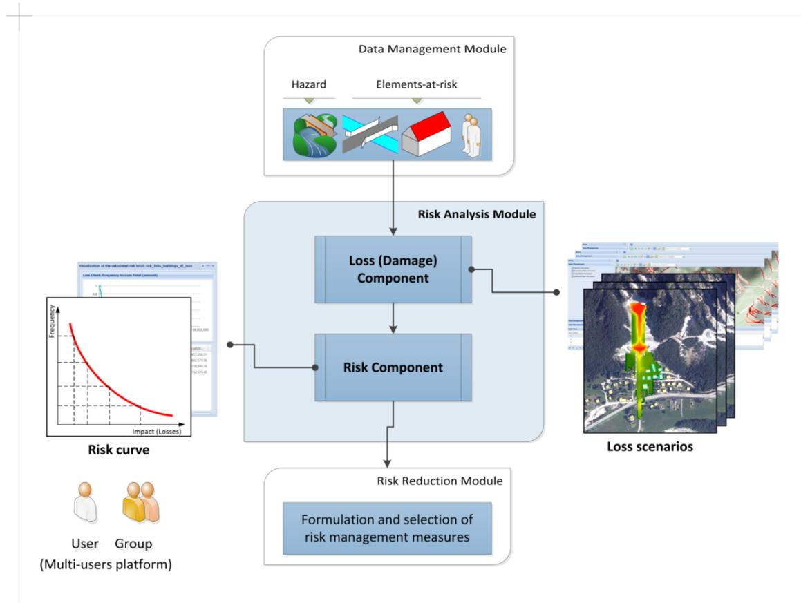
Figure 4.1. Overview diagram illustrating the main modules of the prototype web-GIS platform. For the user interactions, the risk analysis module is mainly intended for expert users (risk managers) while various stakeholder groups can be involved in the risk reduction module for the decision-making process in the formulation and selection of different risk management measures.
