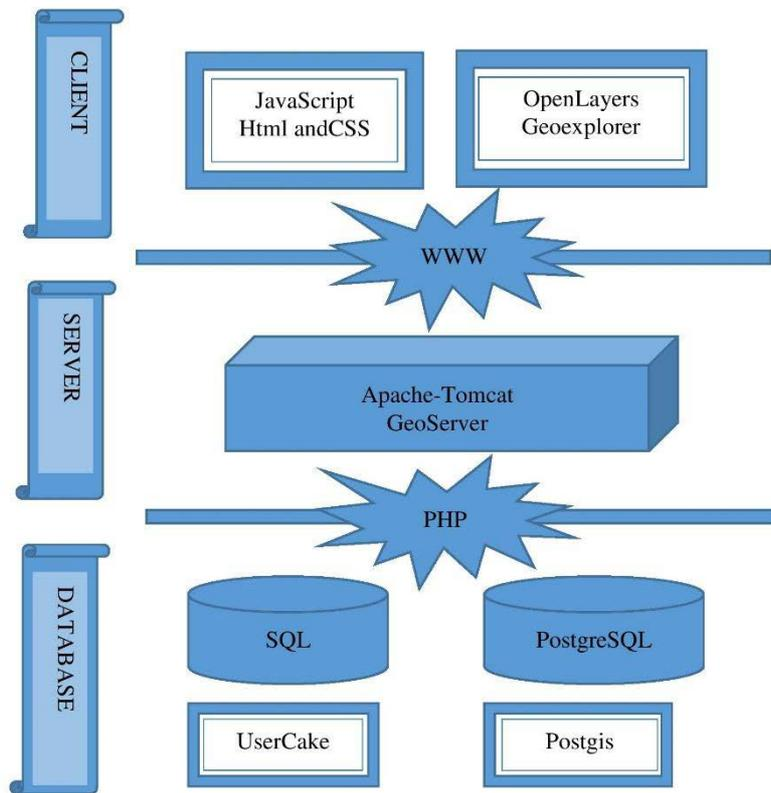
Figure 3 Architecture of the Web-GIS platform
