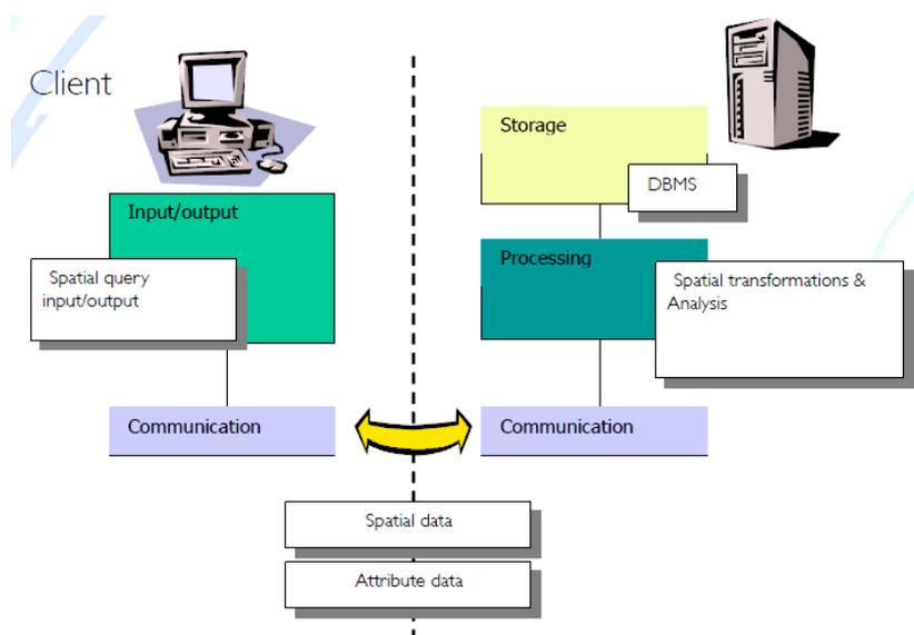
Figure 3.4. A schematic diagram of the server-side processing approach (Source: Kobben et al, 2010).
