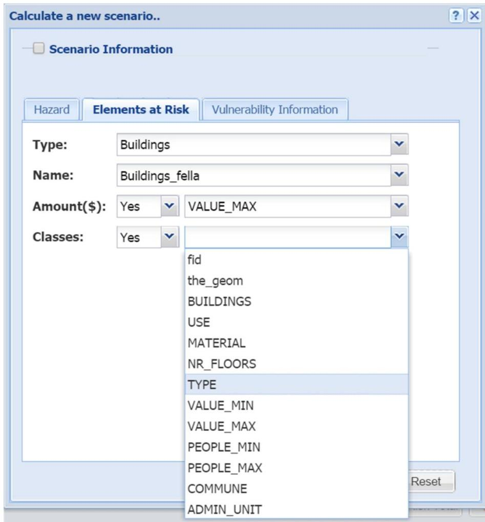
Figure S5. The interface of the loss component illustrating the selection of elements-at-risk input parameters for calculation of a loss scenario. The user can select an existing elements-at-risk map depending on the selected type (e.g., buildings). If available, the user can enter additional information such as amount (e.g., building value) and class (e.g., material type), by querying attribute information of the selected elements-at-risk layer.
