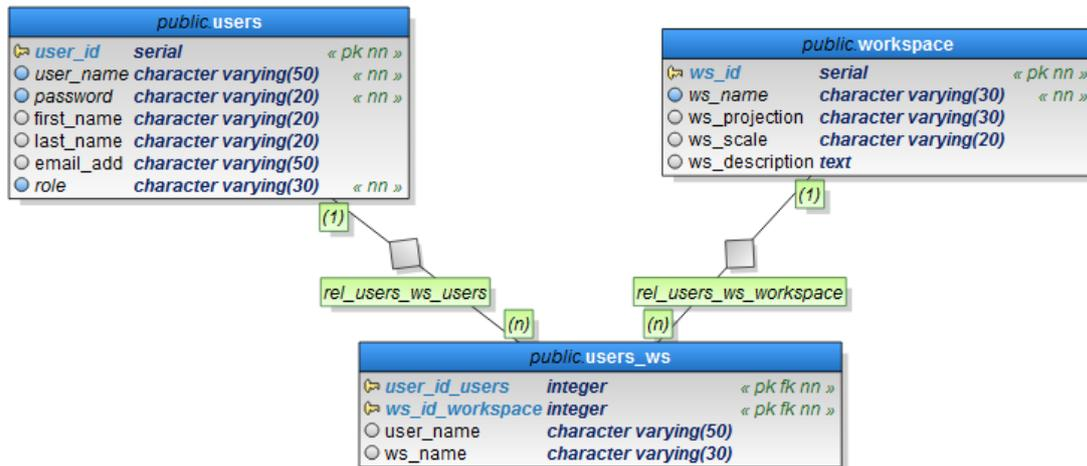
Figure 4. Data model of the public schema.
