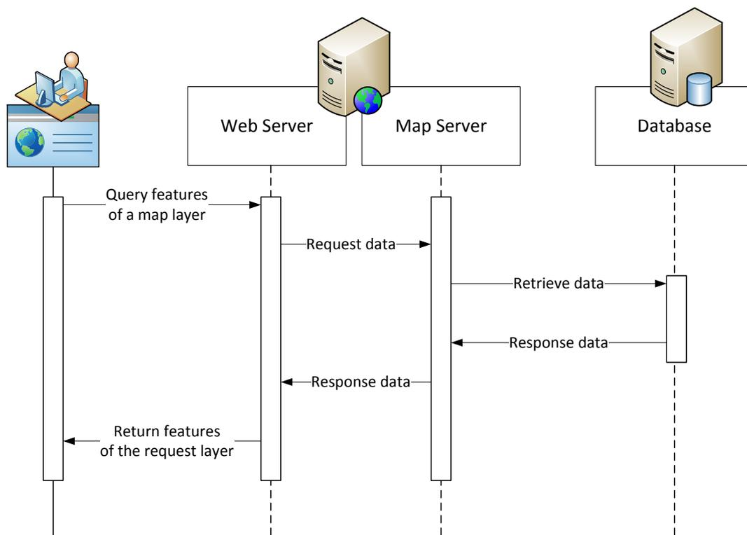
Figure 3.7. A diagram illustrating the communication between client and server components upon the user request to retrieve features of a map layer from the client side.
