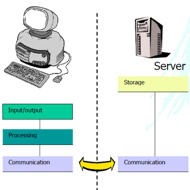
Figure 3.5. A schematic diagram of the client-side processing approach (Source: Kobben et al, 2010).
