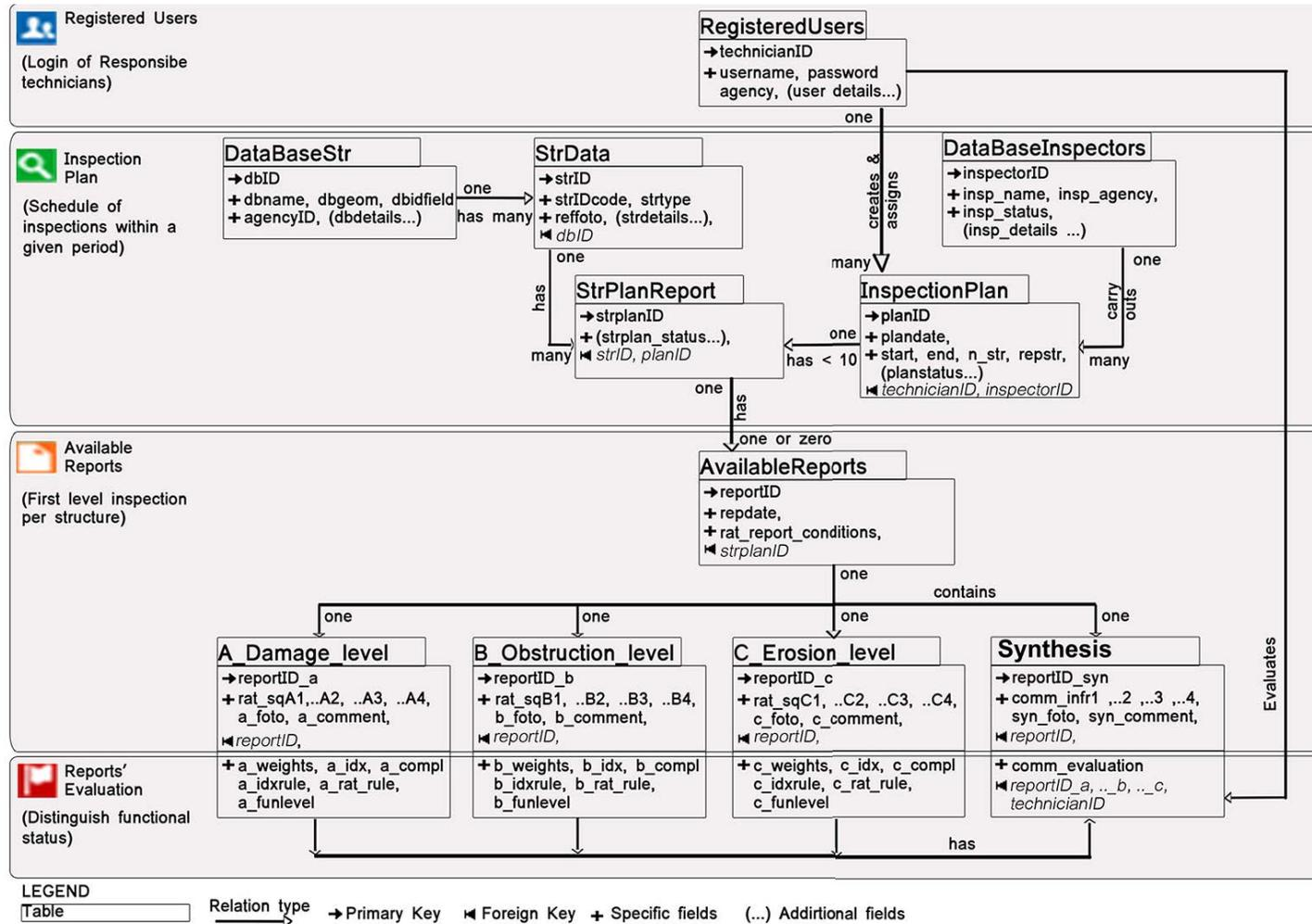
Figure A.1: Conceptual design of the data model behind the web-based application
