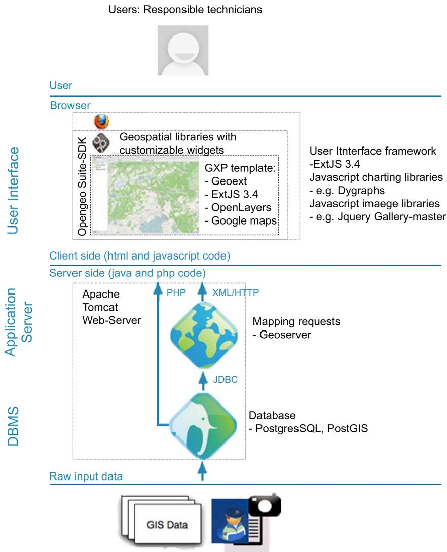
Figure 3: System architecture of the web-GIS platform based on Opegeo Suite. \*Volunteer icon (Civil Protection of FVG region, Italy)
