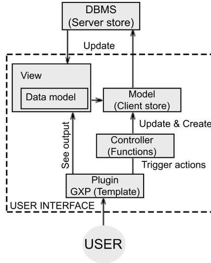
Figure 4: MVC components and illustration of the local client and server stores (adapted from Sencha, 2014)
