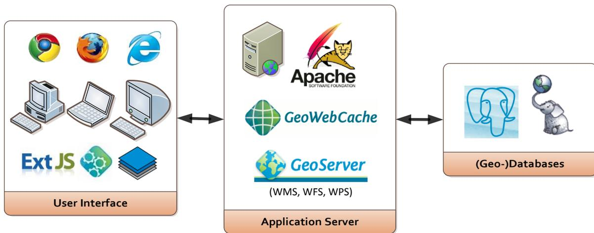
Figure 5.5. Open-source software stack of the prototype.
