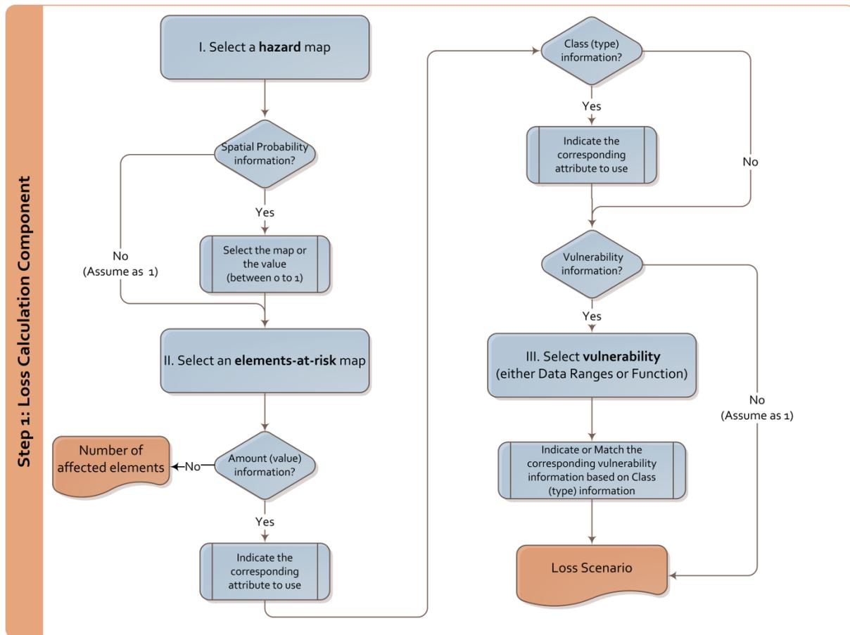
Figure 4.5. Workflow of the loss calculation component, illustrating the three main types of input information (hazard, elements at risk and vulnerability) with additional parameters for the generation of loss scenarios. For example, if the buildings (as elements at risk) have no amount (monetary) information, only the affected number of buildings can be obtained.
