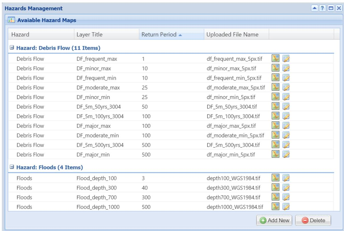
Figure 1. The user interface of a grid panel which shows the list of all uploaded hazard layers in a certain workspace.
