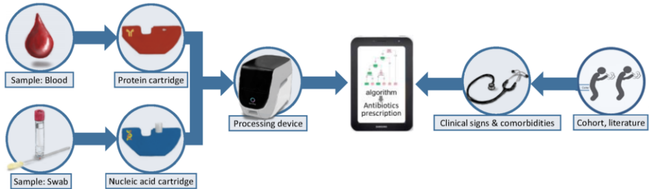
Figure 1. Diagnostic workflow of the proposed POC platform. The nucleic acid cartridge detects RTI infectious agents and resistances via RT-PCR. The protein cartridge detects PCT with bead-based immunoassay. The platform integrates a clinical algorithm as decision support to enable patient management.
