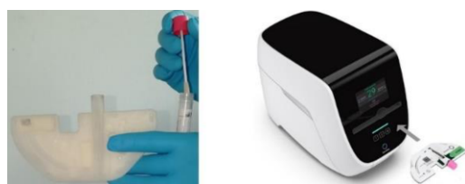
Figure 2. Left: A swab is inserted into the LabDisk PCR-cartridge. Right: The cartridge is inserted into the compact, portable Spindiag Rhonda instrument (20 x 40 x 28 cm).
