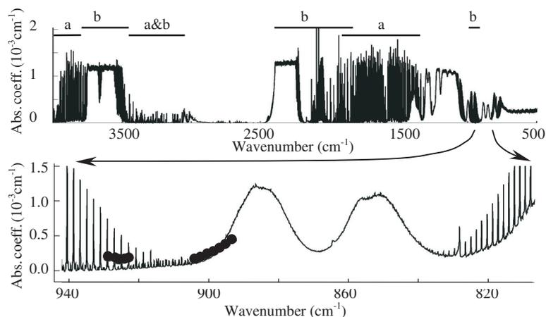
**Fig. 1.** FTIR overview spectra of smoke sample. The PA data taken with the  $^{13}\text{CO}_2$  laser PA spectrometer are shown as dots ( $\lambda$ ). The letters **a** and **b** denote  $\text{H}_2\text{O}$  vapor and  $\text{CO}_2$  absorption, respectively. The origin of the two broad peaks between  $840$  and  $900\text{ cm}^{-1}$  is still unknown.
