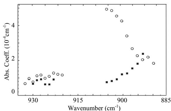
**Fig. 2.** PA spectra of smoke samples (o and ■) taken during electro-knife laparoscopic colorectal surgery during operations on two different patients.
