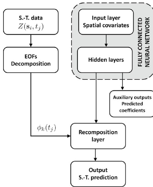
**Figure 1.** The architecture of the proposed framework. The temporal bases are extracted from a decomposition of the spatio-temporal signal using EOFs. Then, a fully connected neural network is used to learn the corresponding spatial coefficients. The full spatio-temporal field is recomposed following Eq. (1) and used for loss minimization.
