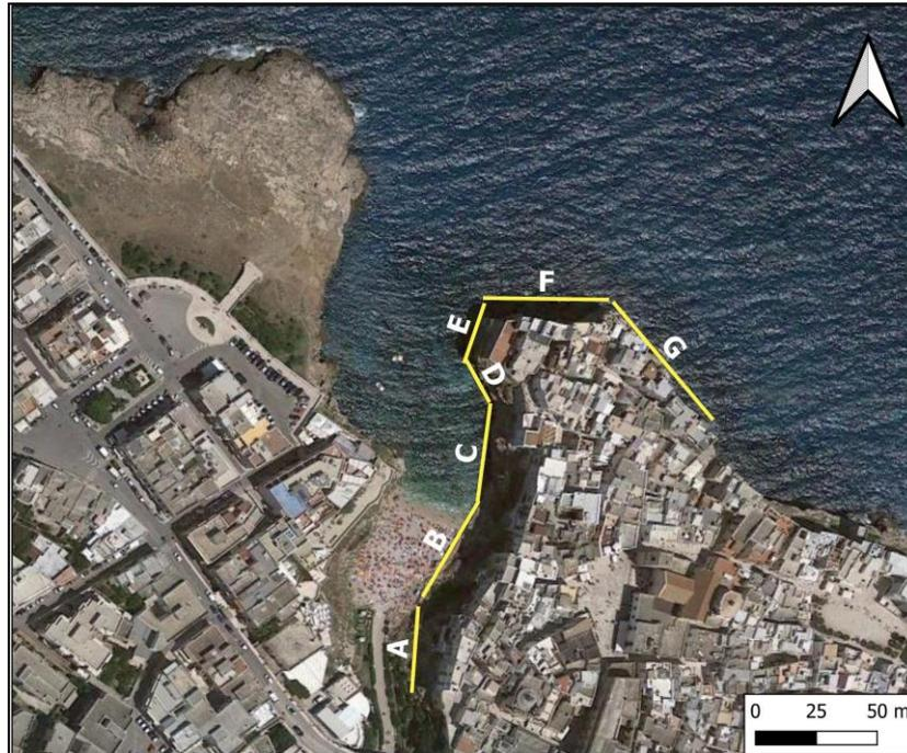
**Figure 7.14:** Subdivision of the study area in 7 sectors, according to the local orientation of the slope, in order to perform the kinematic analyses.
