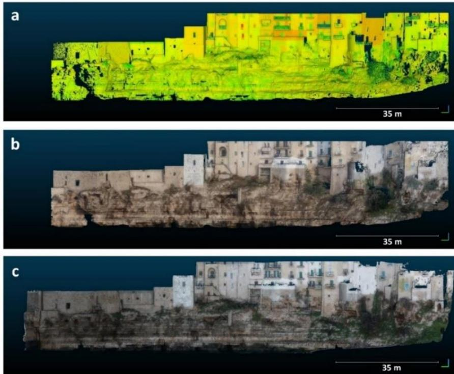
**Figure 4.2:** Final point clouds acquired by means of remote sensing techniques: (a) Terrestrial Laser Scanning point cloud (24,196,954 points and 6852 points/m<sup>2</sup> density); (b) Terrestrial SfM point cloud (6,701,071 points and 1507 points/m<sup>2</sup> density); (c) UAV-SfM point cloud (21,849,920 points and 5244 points/m<sup>2</sup> density).
