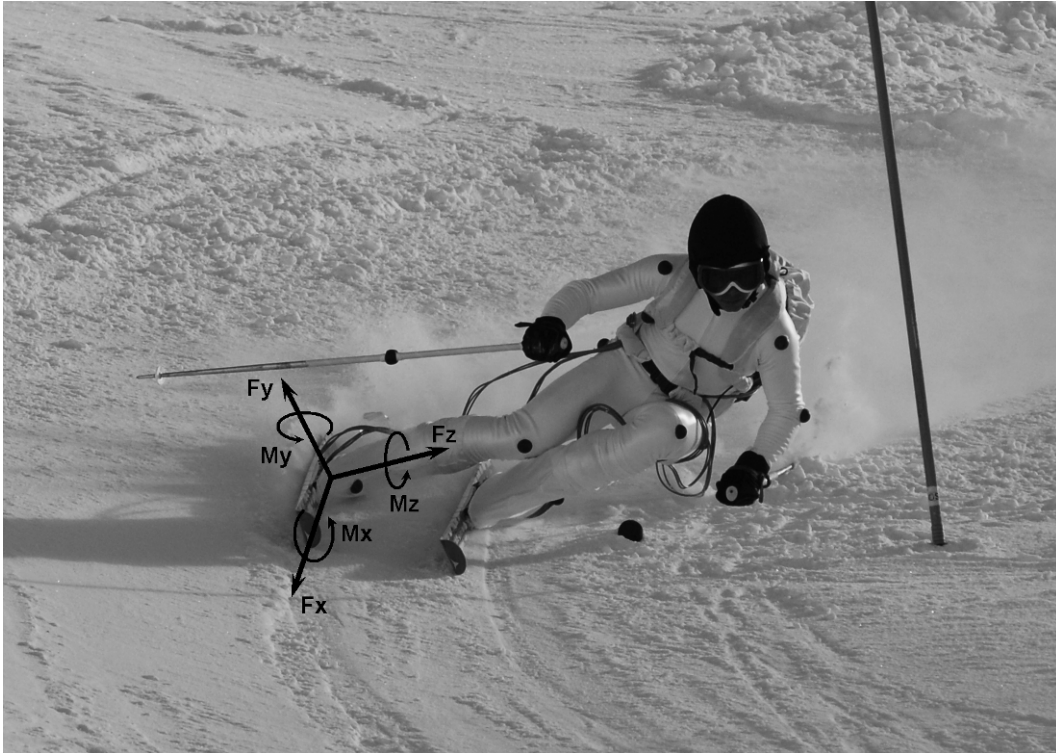
Figure 11-1: An athlete in the giant slalom equipped with the platforms and the backpack. The referential of the right force platform is also represented.
