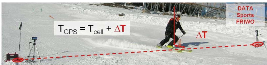
Figure 10-7: Timing cells versus virtual timing derived from GPS .
