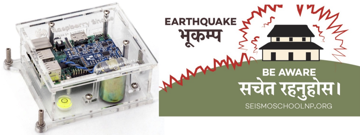
Figure 5.3: Left: The Raspberry Shake 1D low-cost seismometer, installed in 22 schools across Central Nepal (Fig. 5.1). Right: Earthquake awareness sticker, as a reminder, in English and Nepali language (artwork of M. Dessimoz). The sticker image is available for download from our program’s webpage: www.seismoschoolnp.org .
