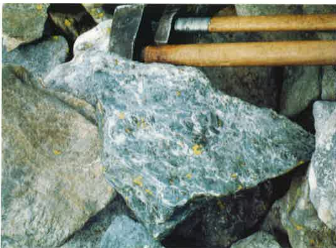
PHOTO 5.1. Mylonitic metagabbros with scattered relics of magmatic hornblende (dark spots within the sample) (sample sv914b) South face of Cima di Bonze, upper Scalario valley, 2370 m.
