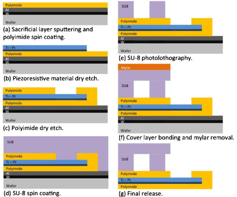
of PI, 2  $\mu\text{m}$  in thickness, is spin-coated and likewise cured. An etch mask of sputtered  $\text{SiO}_2$  (500 nm) is deposited onto the sandwich structure and then patterned by reactive ion etching using a photoresist etch mask. This oxide layer is then used as hard mask during
