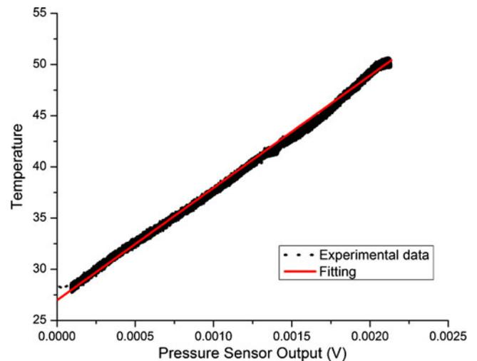
**Fig. 11** Polyimide/SU-8 gauge pressure sensor response to changes in ambient temperature as a function of the voltage output of the gauge pressure sensor and corresponding linear regression fitting to the data
