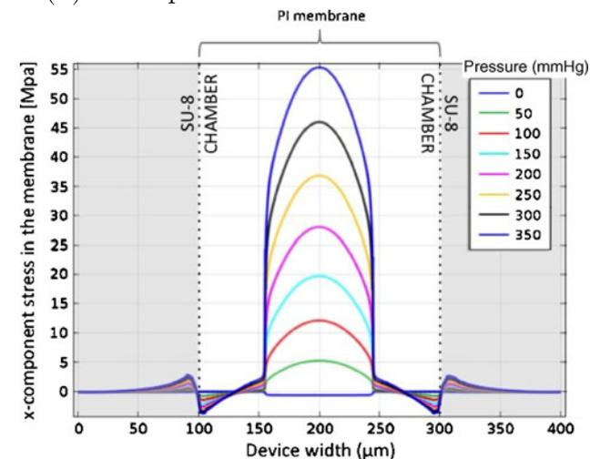
**Fig. 5** x-component of the membrane (a) strain and (b) stress with the applied pressure, in the transverse plane situated at 2  $\mu\text{m}$  from the *bottom* of the PI membrane and along the device width. 2D model including the defined platinum line embedded into the polyimide membrane
