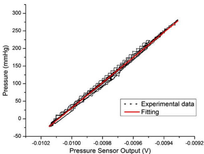
**Fig. 10** Polyimide/SU-8 gauge pressure sensor calibration curve showing reference pressure as a function of the voltage output of the gauge pressure sensor and corresponding linear regression fitting the data
