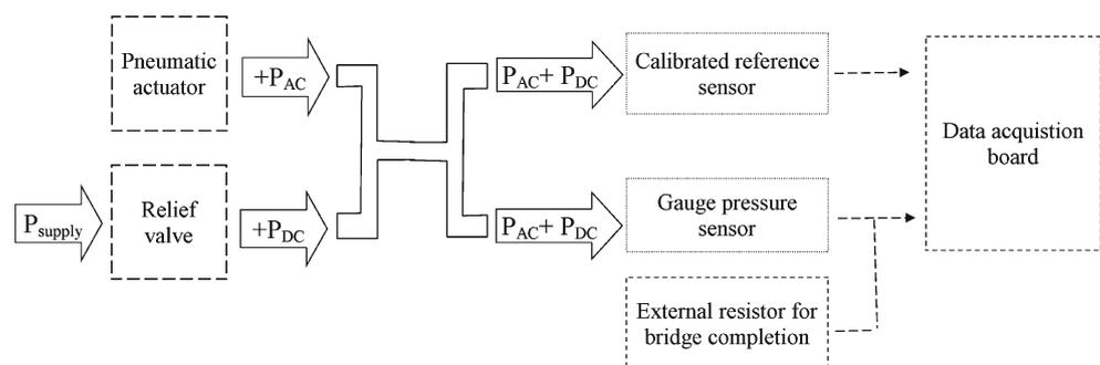
(ENTRAN Pressure Transducer, Model EPX-N01-0.7B) is also attached to the experimental setup and used as reference sensing element for calibrating the device. The reference pressure sensor is powered with 10 V and the signal is acquired using the National Instruments electronic interface previously described, and adding a full-bridge input channel (SCC-SG24). The signal conditioner's gain and span controls for both sensors are set to obtain a full-scale electrical output signal.
